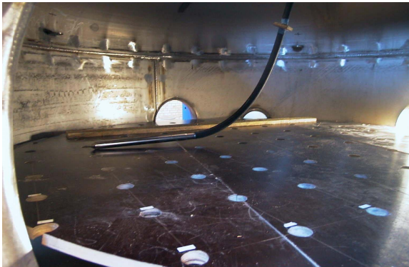
(a) Deck and rod vibrator inside pressure tank.
