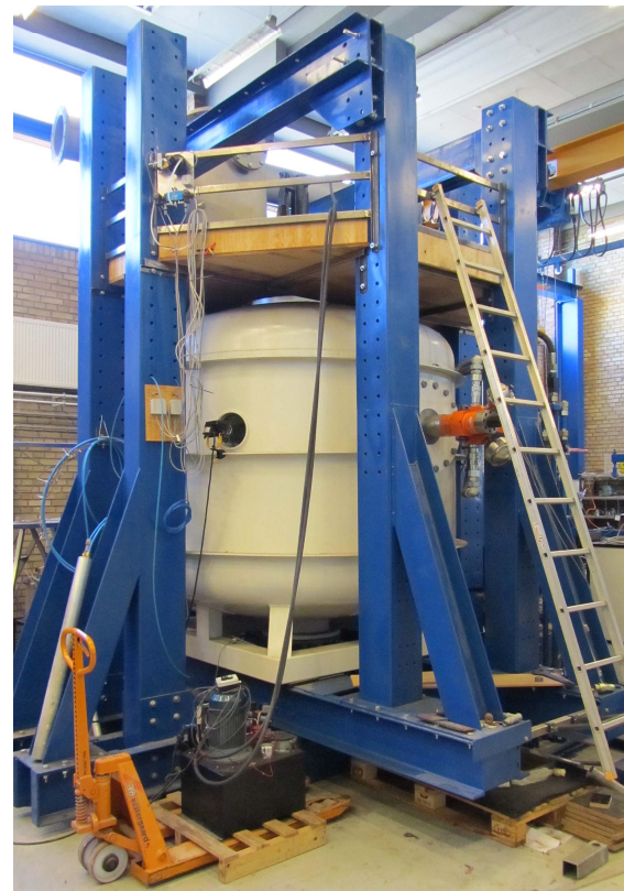
Figure A.2: Image of pressuretank with loadframe.
