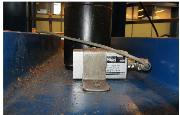
(b) Wire transducer, at the top of the tank.
