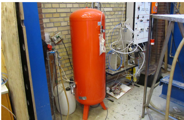
(a) Compressed air container, connected to the pressure tank.
