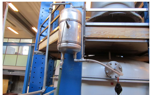
(b) Buffertank, and inlet to pressure tank.
