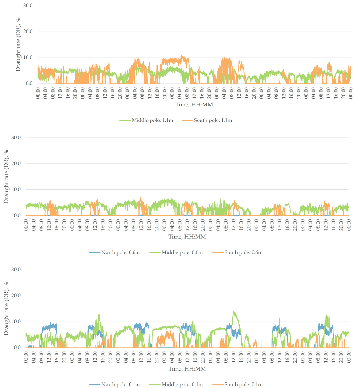
Figure 7.1: North, Middle and South pole draught rates at different height from the ground (Occupied zone) in the Test room. (24-30.07.2023; All hours)
