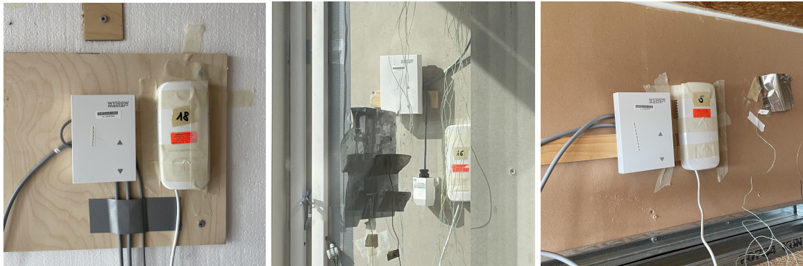
Figure 9.12: IC-meters placement during the WindowMaster validation. Test Room (Right), DSF cavity (Middle) and DCV cavity (Left).
