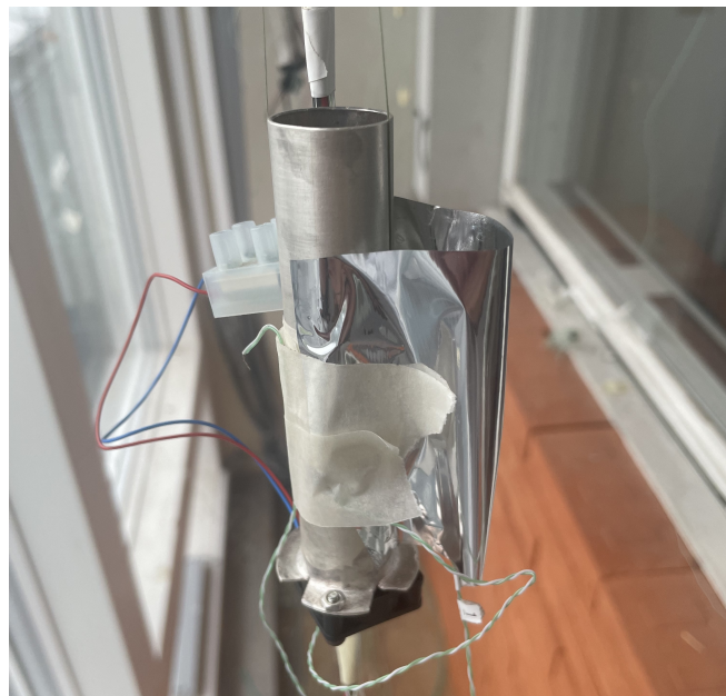
Figure 9.15: Experimental setup of measuring the performance of thermocouples with different types of protection against solar radiation.
