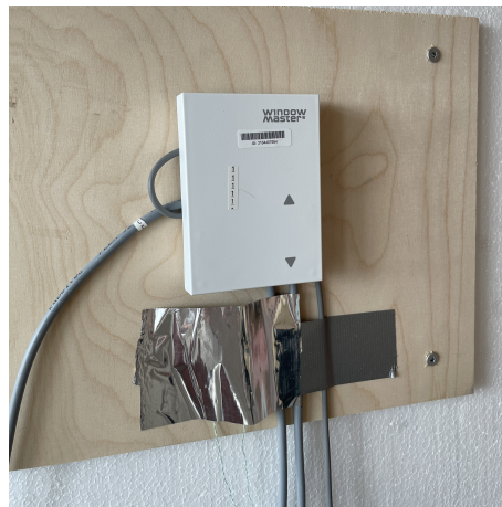
Figure 9.10: K-type thermocouple placement during the WindowMaster validation in the Test Room.
