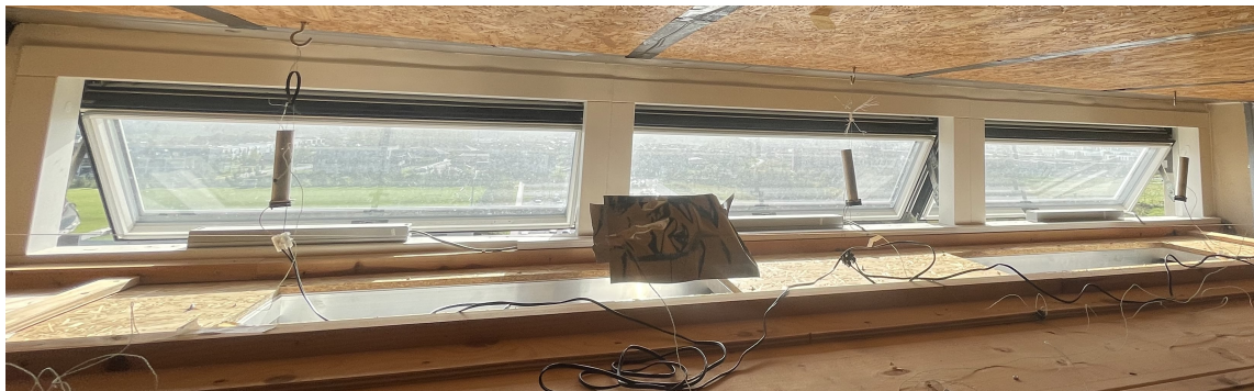
Figure 5.27: Thermocouples located at the bypass area. (The picture serves as a reference for the thermocouple location, and the open state of the windows should be ignored as it was taken within the cooling mode.)
