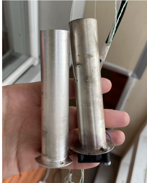
Figure 9.18: Polished (left) and unpolished (right) silver tubes.
