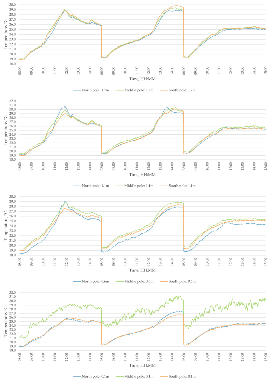
Figure 9.68: North, Middle and South pole air temperatures at 0.1m, 0.6m, 1.1m and 1.7m from the ground (Occupied zone) in the Test room during the occupied hours. (30.11.2023-06.12.2023; 8:00-15:00)
