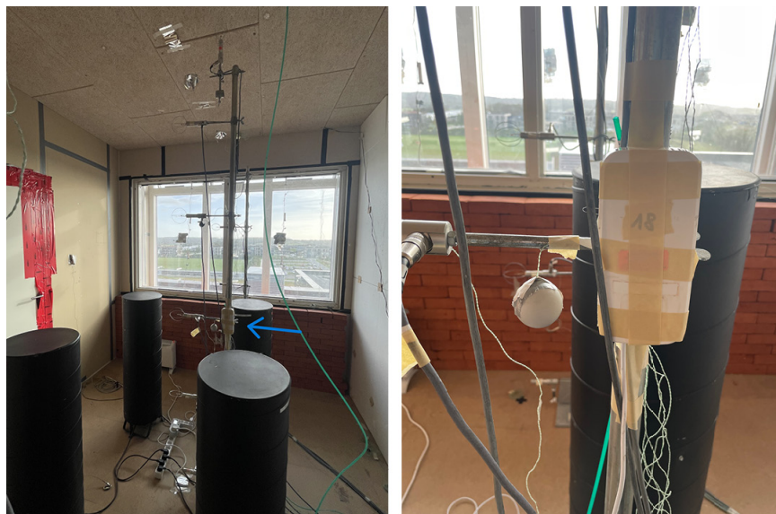
Figure 3.8: In the Test Room, an IC-meter device is used to measure the relative humidity.
