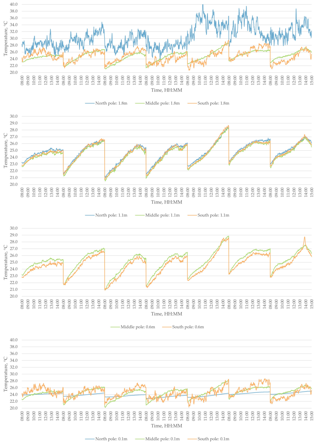
Figure 9.63: North, Middle and South pole air temperatures at 0.1m, 0.6m, 1.1m and 1.7m from the ground (Occupied zone) in the Test room during the occupied hours. (24-30.07.2023; 8:00-15:00)
