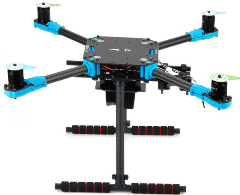
Figure 5.1: Holy Bro X500 V2 ARF kit assembled where the platform board is on the right side of the body.
