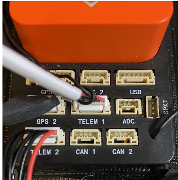
Figure 8.8: Picture of accessible ports on the Cube Orange+ carrier board. RX and TX are connected through the TELEM 1 port
