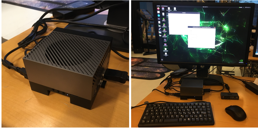
Figure 3.3: The Jetson AGX Orin and its desktop setup, which included a monitor, keyboard, mouse and an external sound card.
