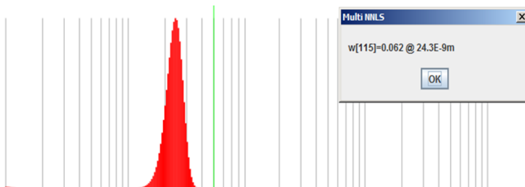
Figure 19: Illustration of a screen shot of a result obtained using CorrelatorComms Software to analyse measurement of 50 nm microbeads. The box on the right of the figure displays a value describing the result. 0.062 is indicative of the relative intensity measured for the sample, and 24.9E-9m is the mean radius of the measured particle sizes.
