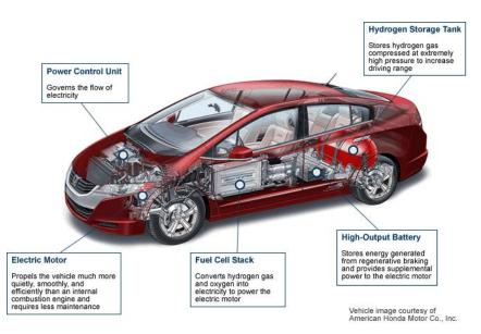
Figure 2.5: Fuel cell vehicle main components [6].
