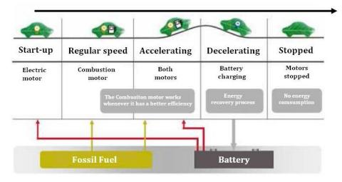
Figure 2.3: Hybrid EV normal behaviour.
