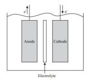
Figure 2.8: Scheme of an electrochemical cell [9].
