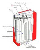
Figure 2.10: Lithium-ion cell of prismatic type [11].
