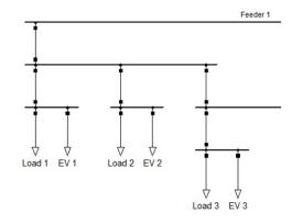
$\label{eq:Figure 4.8: End users and Electric Vehicle model in DIgSILENT PowerFactory software.$
