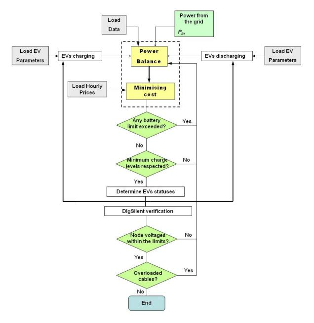
Figure 3.3: Flowchart for the second algorithm.
