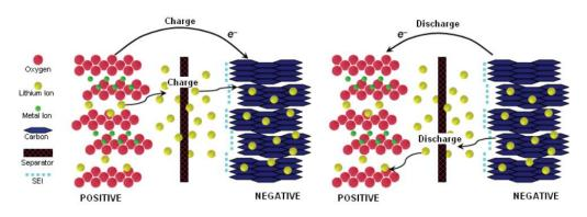
Figure 2.11: Representation of lithium-ion reaction mechanism [12].
