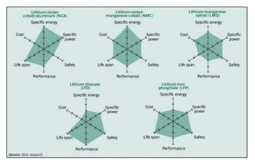
Figure 2.9: Tradeoffs among the five principal lithium-ion battery technologies [10].
