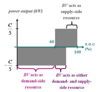
Figure 4.1: Functioning of the battery according to the energy stored [16].
