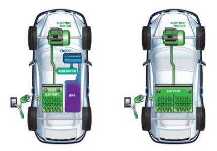
Figure 2.4: Hybrid EV (left) and Battery EV (right) diagrams [5].
