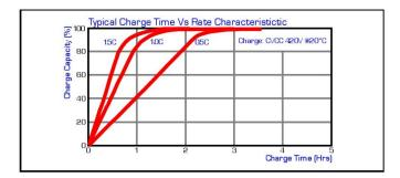
Figure 2.12: Lithium-ion rechargeable battery charging characteristics with different charging rates [11].
