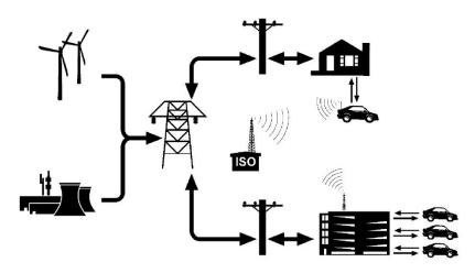
Figure 2.6: Power lines and wireless control connections between V2G and the grid [7].
