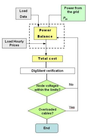
Figure 3.2: Flowchart of the first algorithm.
