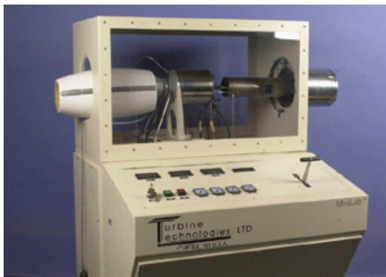
*Figure 6.1: The SR-30 Turbojet Engine modelled in this project [Technologies, 2007].*
