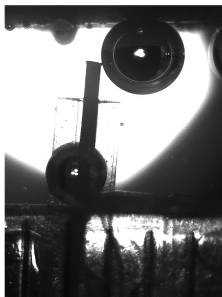
**Figure 4.17:** Air bubble on the bottom of a reference filter submerged in water. The contact angle is the receding angle as the volume is increasing at this point.
