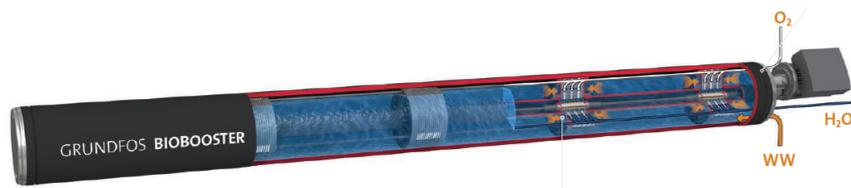
**Figure 1.2:** Model of the Grundfos BioBooster MBR. The compartment to the left contains the activated sludge used to biologically treat the wastewater. Next there are cross flow impeller fans to reduce fouling, and to the right the filters are located. [4]
