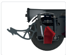
Retracted and extended mouth piece.
