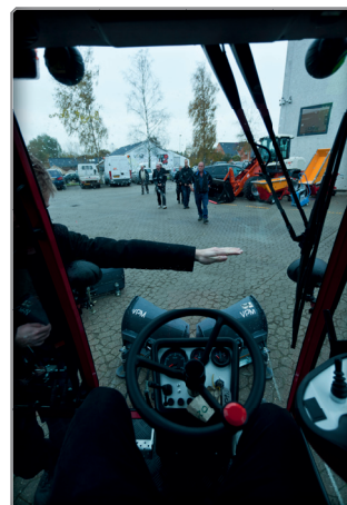
Demonstration of how low the tools are in the field of vision through the window. Arm located approximately half way up.
