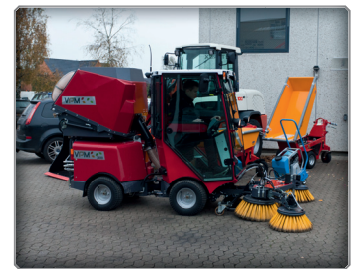
When driving faster, the VPM 3400 has a tendency to bob back and forth due to the short wheel base and suspension.
