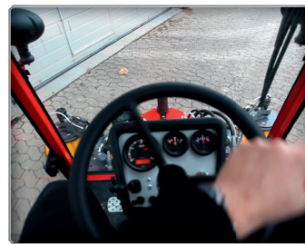
Limited vision of the tools during operation of street sweeper attachment.
