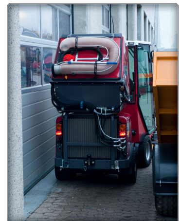
Manoeuvring the VPM 3400 in a tight spot is quite possible, however the protruding mirrors have a tendency to collide with walls, etc. causing misalignment.
