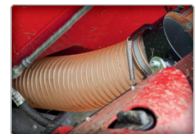
Example of flexible hose, currently used all the way from the mouth piece to the vacuum box.
