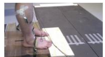
Figure 2 - The MVIC experimental setup (the MVIC block is seen from the top). The feet were fixed with straps and the toes placed on the MVIC platform.
