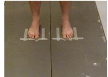
Figure 1 - Tape markings on the two forceplatforms, with five centimeters between each marking.
