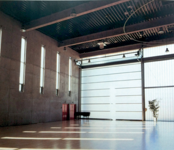
Fig.12. Multipurpose hall with the openable end wall in semi-transparent fibreglass connecting the space with the outdoor when opened for concerts, markets, outdoor cinema, etc.
