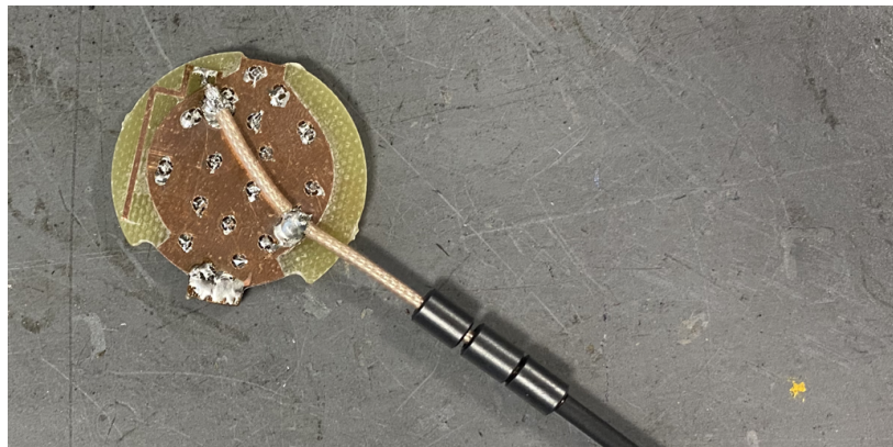
Figure 6.11: Printed MIFA PCB with the negation of pigtail effect in the form of ferrite beads and soldering points.
