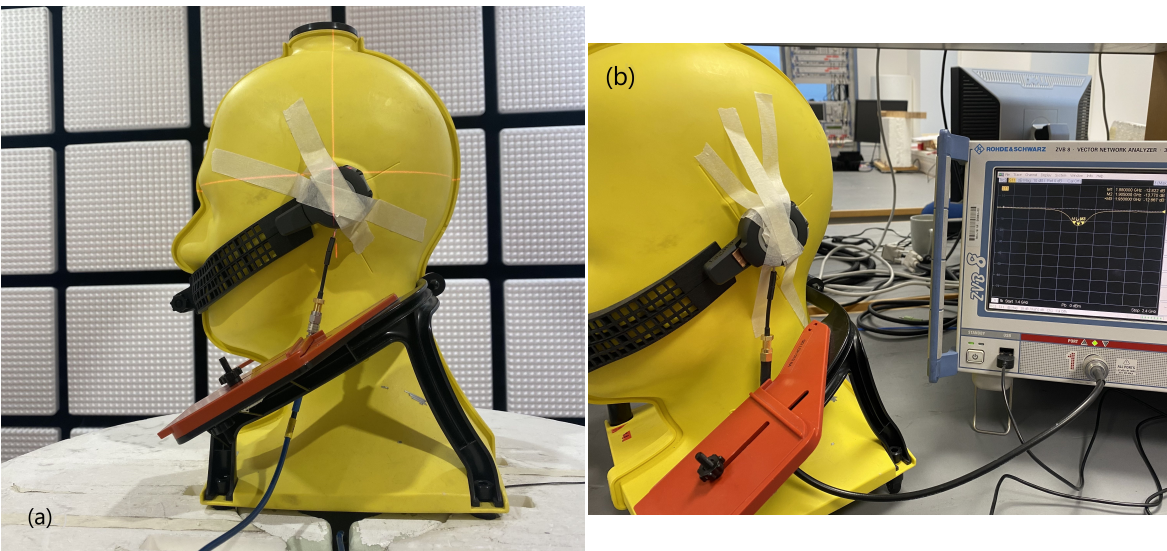
Figure B.17: The test setups for measuring the ground extension effect. This test is solely in head coupling configuration. The figures show the measurement setup in the Stargate and when measuring using a VNA.
