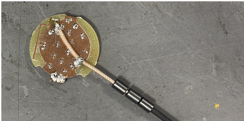
Figure B.1: Soldering setup of the RF pig tail on the DUT for measurements.
