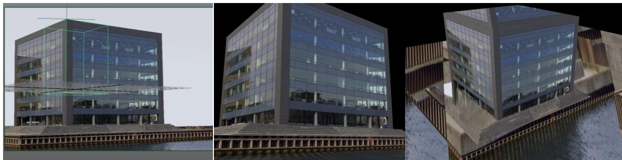
Figure 6 On the Left: Original picture with aligned geometry. Centre: Projected texture. Right: Limits of camera projection.
