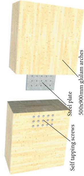
Because of transportation problems the arches must be divided into several pieces. They will be connected together in a way where a steel plate is placed between the laminates and then attached together with self tapping screws.
