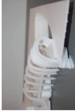
Shape experiment where the bridge consist of glulam arches that have the same height through the whole bridge, and where the arches go down and meet the landscape.
