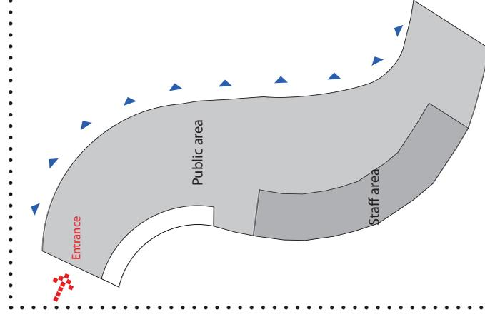
Floor plan with entrance at the end of the building. A clear line is kept through the whole building and the view possibility is in focus.
