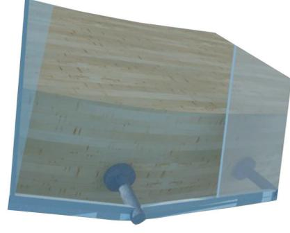
connected to steel pins that will be attached to the glulam arches. This way the attachment of the glass won't be disturbing and it is not necessary with some extra structure to carry the glass. The glass will also get some distance from the glulam arches, and this way the arches will be in a protected environment.
