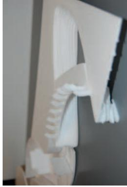
Shape experiment where the bridge consist of glulam columns that are cut in the same height. The idea is that they should have the same curve as the arches.
