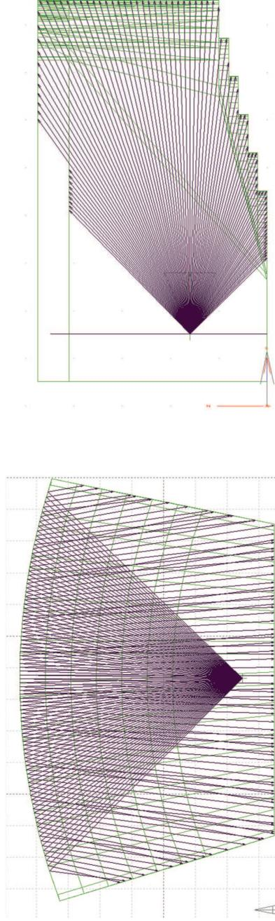
Figure.: These figures display how the sound is distributed in the room
