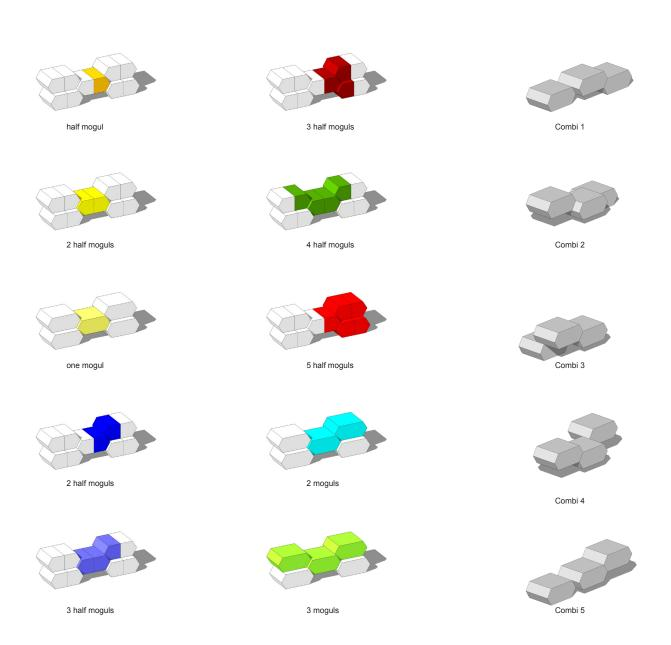
By extruding in depth and letting the moguls step downwards it creates an interesting interplay in the structure. It also make spaces between each mogule, which has the potential of being outdoor areas and balconies. When connecting the moguls by its angled edge, the structure will be pushed down resulting in a half storey structure, which can be troubling when entering the moguls from the back.
