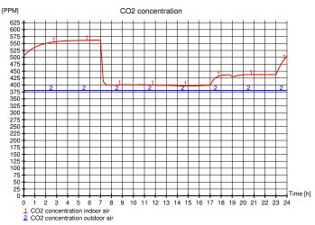
The  $CO_2$  concentration stays well below 800 and max at 562PPM at 7am just before the ventilation system goes into operational hours.
