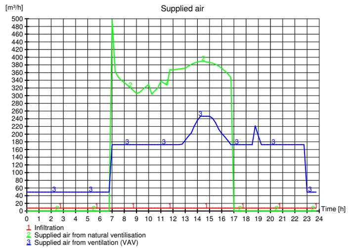
Between 7am and 5am most of the supplied air comes from natural ventilation. The rest of the day only mechanical ventilation is used.
