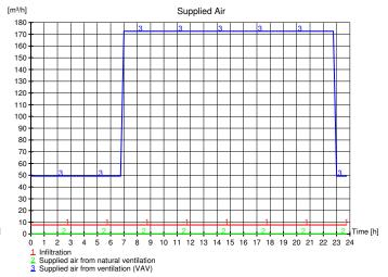
There is no natural ventilation during winter time. The mechanical ventilation has operation hourse between 7am and 11pm, but is always running.
