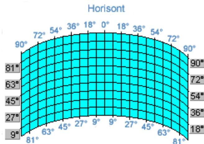
This diagram shows the amount of the horizon that is covered by mountains or other buildings, the blue dots is the clear sky and the black dots are area covered by obstacles.
