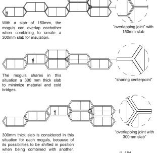
300mm is used to be sure that this thickness is kept in cases where the edges of the moguls doesn't interacts with eachother. When met the slab will be 600mm, which is considered too be overuse of material.
