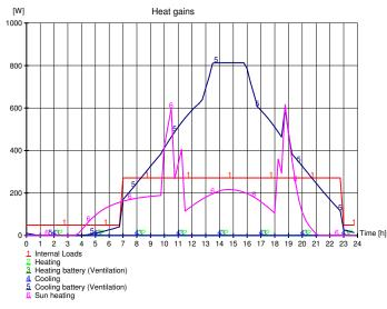
The sun, internal loads and cooling batteries from ventilation is the heat gain sources during summer. Heating and heating batteries are not active in summer time.
