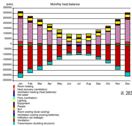
This diagram shows the monthly heat balance of each post. This is useful to see where the heat is gained from, and by which mean its lost. It shows that most heat is lost from ventilation, while most of the heat gain is from the ventilations heat recovery.
