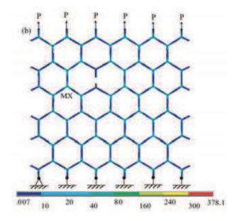
When one tube in the honeycomb structure is broken, the surrounding arms can easily carry the load due to the structure's ability to transfer forces. The colors show the von Mises stress distribution, with dark blue as lowest stress and MX referring to the place with maximum stress. Image credit: Xiong Zhang, et al.
