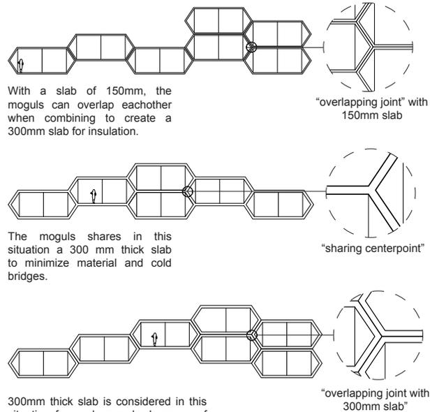
With a slab of 150mm, the moguls can overlap eachother when combining to create a 300mm slab for insulation.
