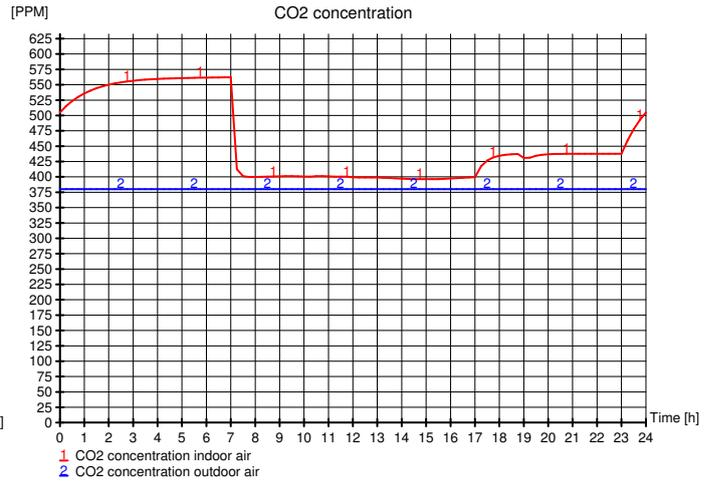
The CO<sub>2</sub> concentration stays well below 800 and max at 562PPM at 7am just before the ventilation system goes into operational hours.
