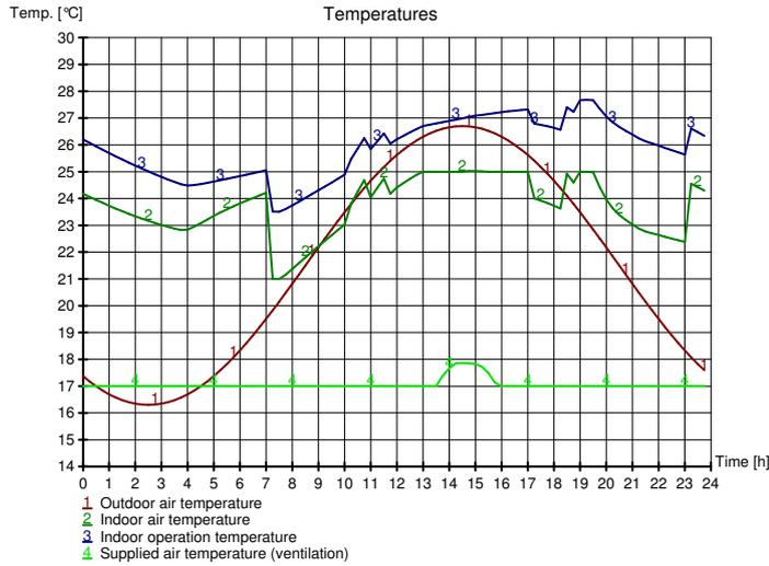
The indoor air temperature never goes above 25 °C and max between 1pm and 8pm.
