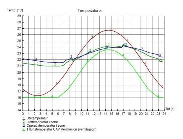
Simulated temperature flow for hotel room at dimensioned summer conditions. [sintef, 2012]
