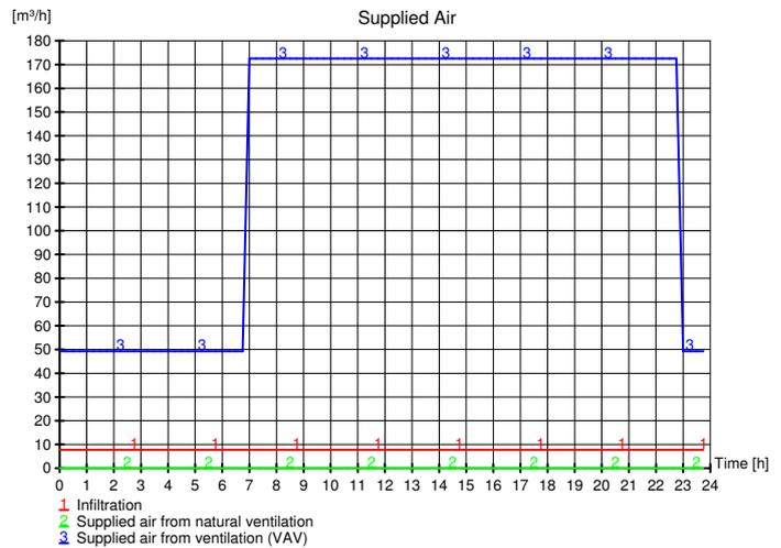
There is no natural ventilation during winter time. The mechanical ventilation has operation hours between 7am and 11pm, but is always running.
