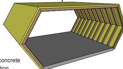
Bottom mogul with concrete floor slab as foundation
