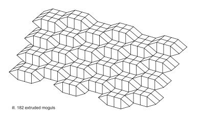
When looking at a section of the grid, it only allows for full height hallways at every second mogul storey, which is caused by the half steps of the structure. This is not an optimal way for the users to enter the different moguls, and a solution for this will be found in the synthesis phase. The flexibility of the moguls also allows rooms to be extended in depth to create larger volumes.
