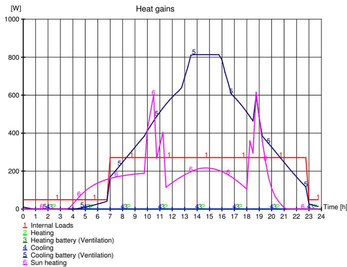
The sun, internal loads and cooling batteries from ventilation is the heat gain sources during summer. Heating and heating batteries are not active in summer time.
