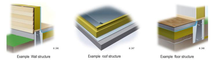
**CONSTRUCTION ELEMENTS** WALL 1 WALL2 WALL3 ROOF 1 ROOF 2 FLOOR1 FLOOR2 ROCK 301 436 329 244 1011 Thickness [mm]: 304 455 320 228 246 300 150 180 Insulation [mm]: 228 160 0.18 0.09 U-value [W/m<sup>2</sup>K]: 0.18 0.15 0.18 0.15 0.09 Wood Mix Wood Massive wood Bearing: Concrete Concrete Concrete Parquet Wood Stone Mix Wood Mix Stone Stone Cladding:
