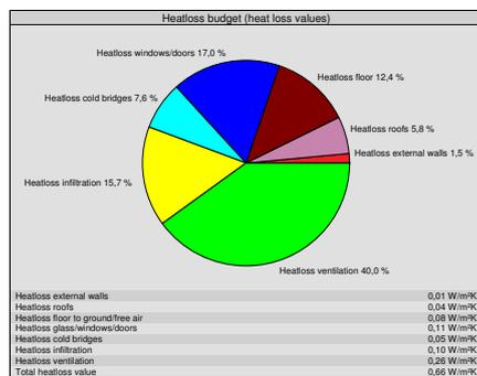
This table and diagram shows the amount and share of each heatloss post. It shows that most of the loss (40%) comes from ventilation. The total heatloss value is 0.66 W/m²K.
