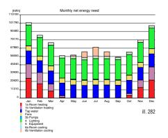
This diagram shows the monthly net energy need of each post. One can see that room heating and ventilation heating is active from October to April, with no room heating in the summer. The ventilation cooling is active only from May to August. Lighting, fans and tap water is active all year long.
