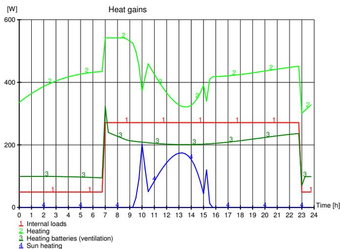
Internal loads, heating, heating batteries from ventilation and sun heating is the sources of heat gains during winter. No cooling is used in winter time.
