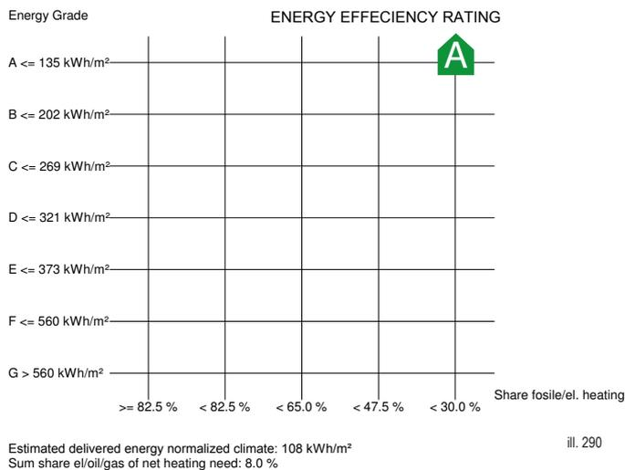
Before adding the geothermal heating, the energy efficiency rating was on B, but after adding it the energy efficiency rating gets an A with 106 kWh/m<sup>2</sup>. The rating is also on the right side of the chart which indicates that it use less than 30% of the energy for heating based on non fossile/el. heating. [Appendix 24].
