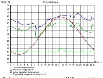
The indoor air temperature never go above 25  $^\circ\text{C}$  and max between 1pm and 8pm.
