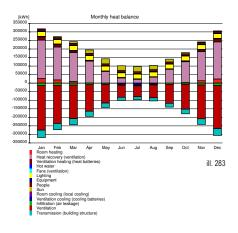
This diagram shows the monthly heat balance of each post. This is useful to see where the heat is gained from, and by which mean its lost. It shows that most heat is lost from ventilation, while most of the heat gain is from the ventilations heat recovery.
