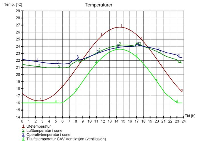
Simulated temperature flow for hotel room at dimensioned summer conditions. [sintef, 2012]
