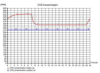
The  $CO_2$  concentration stays well below 800 and max at 559PPM at 7am just before the ventilation system goes into operational hours.
