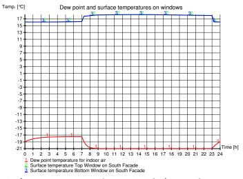
Surface temperature windows: Min 16 °C / Max 18 °C Dew point temperature indoor: Min -21 °C / Max -17 °C
