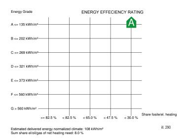
Before adding the geothermal heating, the energy efficiency rating was on B, but after adding it the energy efficiency rating gets an A with 106 kWh/m<sup>2</sup>. The rating is also on the right side of the chart which indicates that it use less than 30% of the energy for heating based on non fossile/el. heating. [Appendix 24].
