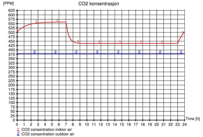
The CO<sub>2</sub> concentration stays well below 800 and max at 559PPM at 7am just before the ventilation system goes into operational hours.
