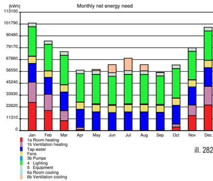
This diagram shows the monthly net energy need of each post. One can see that room heating and ventilation heating is active from October to April, with no room heating in the summer. The ventilation cooling is active only from May to August. Lighting, fans and tap water is active all year long.
