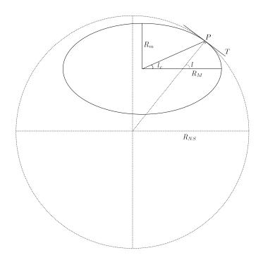
Figure 3.3: The earth and its radius of north-south curvature at P
