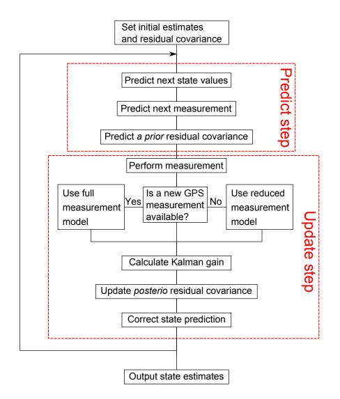
Figure 6.2: An overview of the estimation filter
