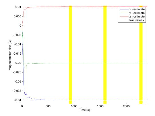
Figure 10.9: The estimated magnetometer biases. The dotted lines are the true constant bias values. The highlighted areas are the GPS outage periods.
