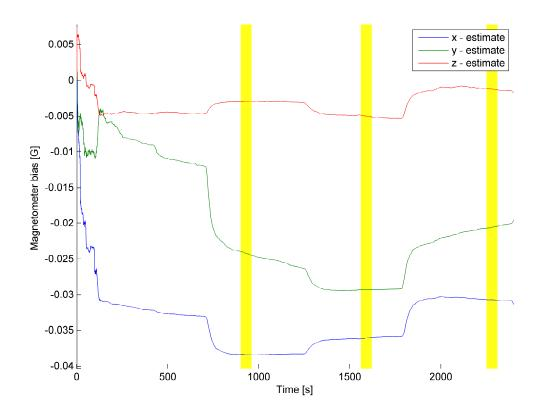
Figure 11.10: The estimated magnetometer bias.
