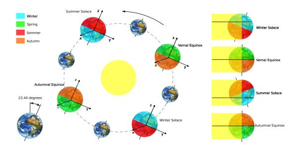
**Figure 2.1:** Earth Centered Initial Reference Frame, which is defined as the Z-axis pointing towards the north pole and X-axis pointing towards the center of the sun, one time each year at vernal equinox [of Electronic Systems 10]
