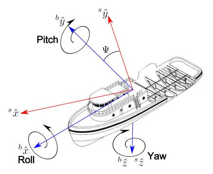
**Figure 2.4:** The HVRF axis, denoted with *b* and the SRF axis, here shown with a misalignment around the Z-axis with a value of  $\Psi$
