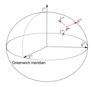
**Figure 2.3:** Navigation Reference Frame, where the X-axis points towards the North pole, and the Y-axis points towards East and the Z-axis points towards the center of the earth
