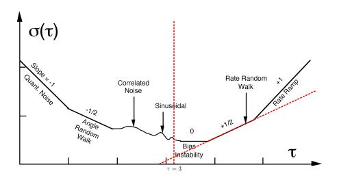
**Figure 4.1:** An example of a typical Allan variance plot [Gyro 97, Appendix C, p. 71] with added dotted lines indicating the procedure of finding  $K_{RRW}$ . The axises here are log-log.
