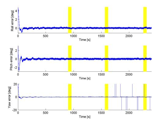
Figure 10.5: The attitude estimation errors. The highlighted areas are the GPS outage periods.
