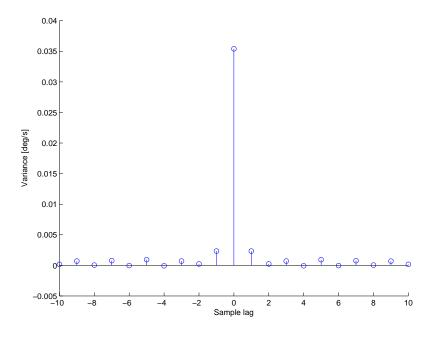
Figure 4.3: Covariance of gyroscope measurement of a 2 min stationary test
