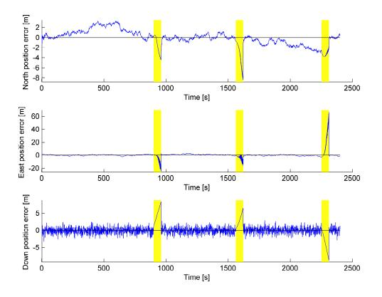
Figure 10.7: The position error of the different NRF axises. The highlighted areas are the GPS outage periods.
