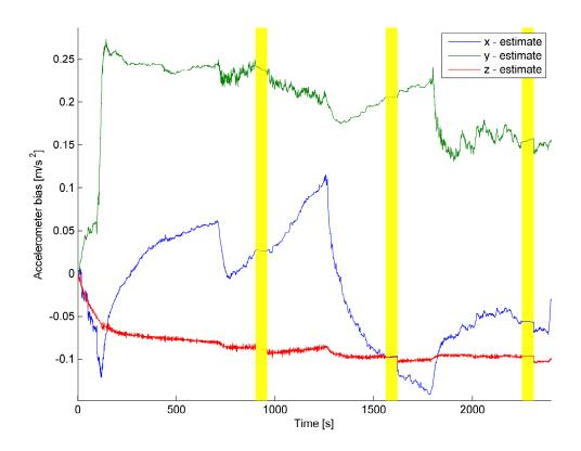
Figure 11.11: The estimated accelerometer bias.
