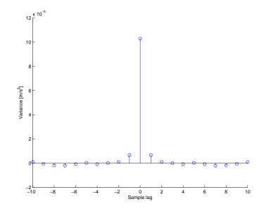
Figure 4.5: Covariance of accelerometer measurement of a 2 min stationary test
