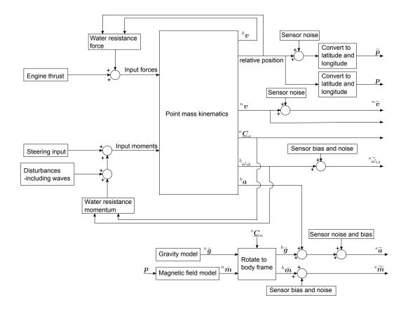
Figure 6.1: An overview of the simulation environment
