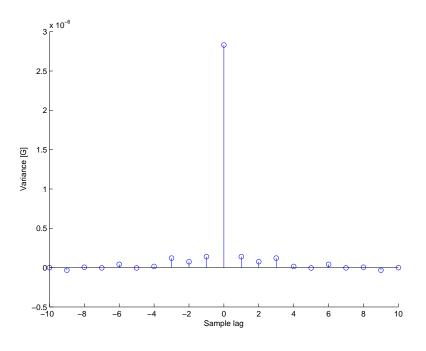
Figure 4.6: Covariance of magnetometer measurement of a 2 min stationary test
