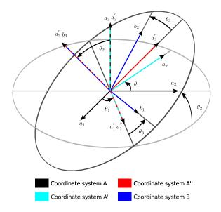
**Figure A.1:** Example of 3-1-3 Euler rotation sequence.  $A \to A' \to A'' \to B$
