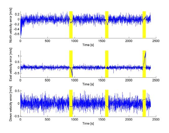
Figure 10.6: The velocity estimation errors of the NRF axises. The highlighted areas are the GPS outage periods.
