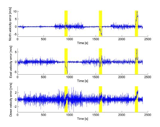
Figure 11.7: The velocity error of the two horizontal NRF axises. The highlighted areas are the GPS outage periods.
