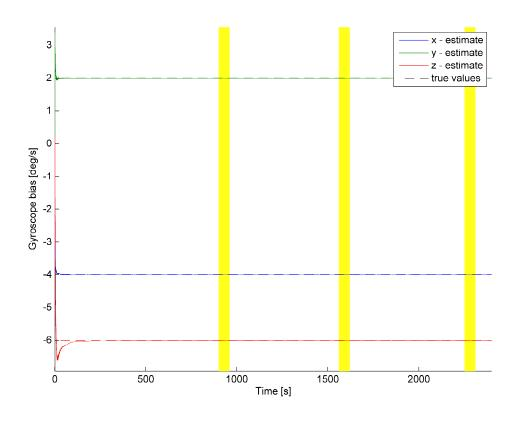
Figure 10.8: The estimated gyroscope biases. The dotted lines are the true constant bias values. The highlighted areas are the GPS outage periods.
