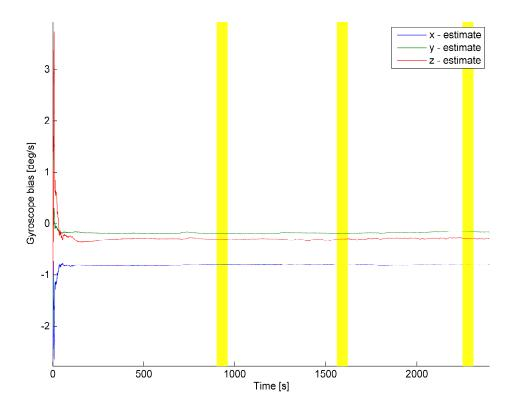
Figure 11.9: The estimated gyroscope bias.
