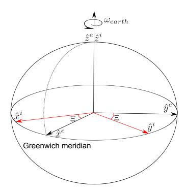
**Figure 2.2:** Earth Centered Earth Fixed Reference Frame, where the Z-axis points towards the North Pole, and the X-axis points towards the Greenwich meridian.
