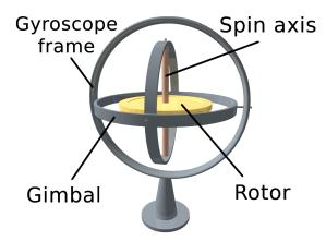
Figure 1.1: Basic gimbaled gyroscope
