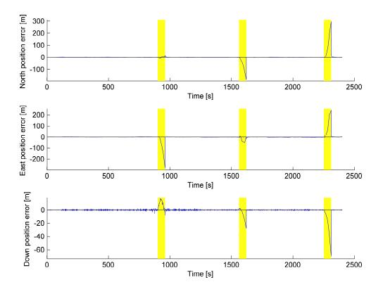
Figure 11.8: The position error of the different NRF axises. The highlighted areas are the GPS outage periods.
