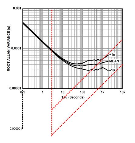
**Figure 4.4:** The Allan variance plot for the IMU's accelerometer [Ana 11] with extended Y-axis together with dotted line indicating the procedure of finding  $K_{RRW_{acc}}$
