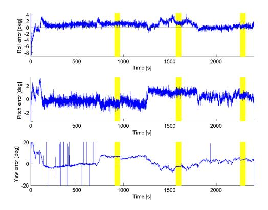
Figure 11.5: Attitude errors. The highlighted areas are the GPS outage periods.
