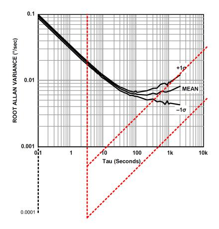
**Figure 4.2:** The Allan variance plot for the IMU's gyroscope [Ana 11] with extended Y-axis together with dotted line indicating the procedure of finding  $K_{RRW_{gyro}}$
