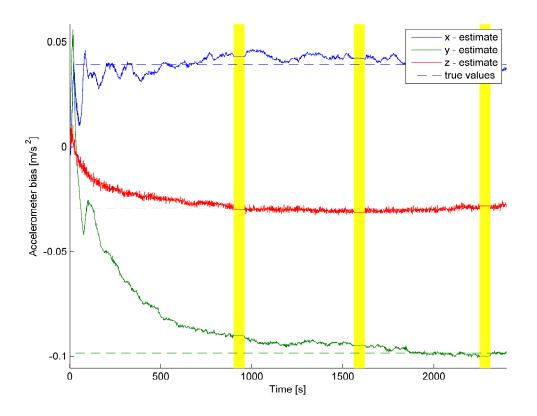
**Figure 10.10:** The estimated accelerometer biases. The dotted lines are the true constant bias values. The highlighted areas are the GPS outage periods.
