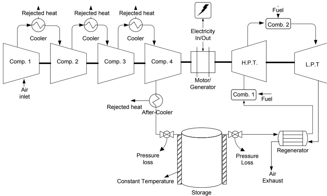
**Figure 4.1:** The schematic diagram of the main CAES plant configuration modeled.
