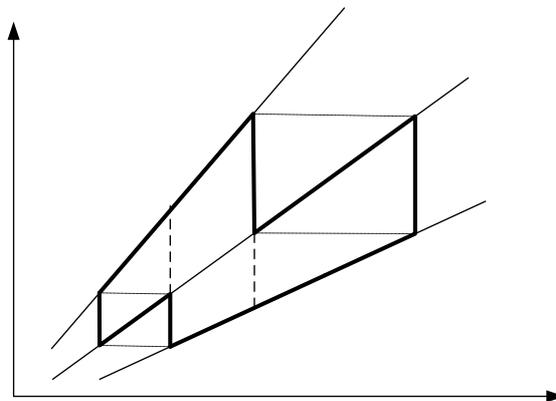
**Figure 3.6:** T-s diagram for an intercool/reheat cycle. The diagonal lines are constant pressure lines.
