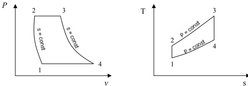
**Figure 3.2:** The P-v and T-s diagrams of a Brayton cycle. Note that the enclosed area represents the net work output from the cycle in both diagrams (Figure note to scale).
