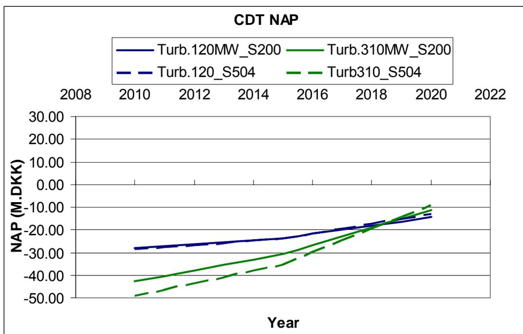
**Figure 5.7:** the Net Annual Profit (NAP) for the Current Day Technology (CDT) for two values of storage size (200,000 m<sup>3</sup> and 504,000 m<sup>3</sup>) and two turbine sizes (120 MW and 310 MW).
