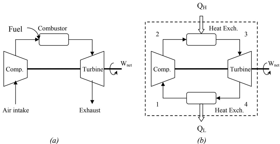
**Figure 3.1:** (a) Simple open cycle gas turbine representation. (b) The standard air cycle representation of the simple cycle.
