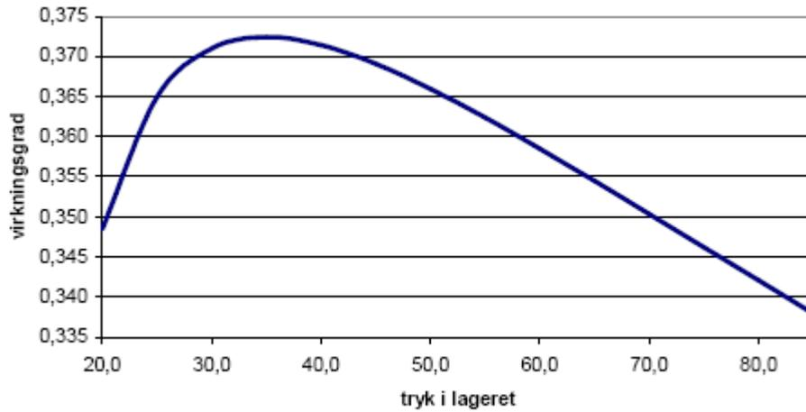
**Figure 3.7:** The GT efficiency of a CAES plant under varying storage pressures (X-axis) found by statistical simulation. (Brix and Szameitat, 2003)
