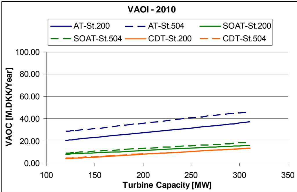
**Figure 5.4:** Variable Annual operational Cost (VAOI) for the year 2010 for various turbine capacities at cavern sizes of 200,000m<sup>3</sup> and 504,000m<sup>3</sup> respectively
