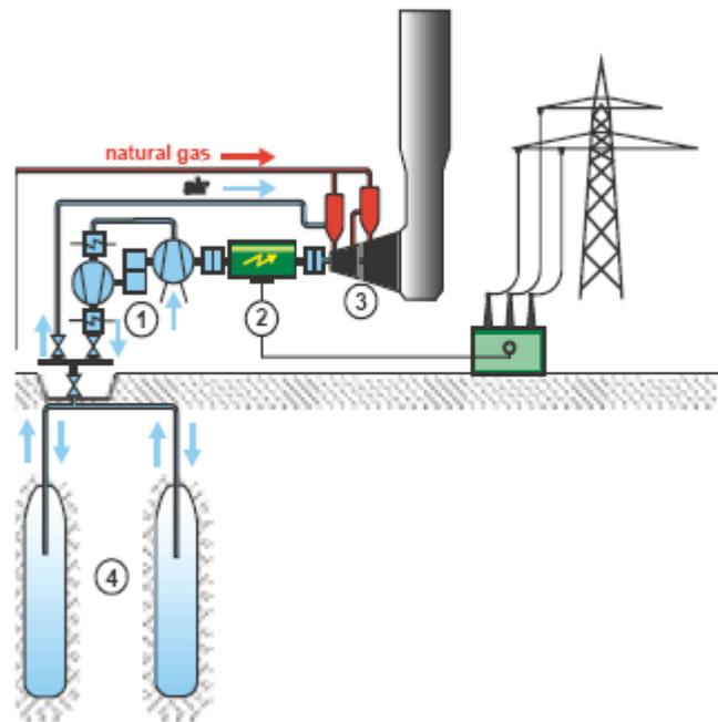
**Figure 3.8:** Schematic representation of the Huntorf CAES plant. Note the 2 stage compression and the single generator/motor unit.
