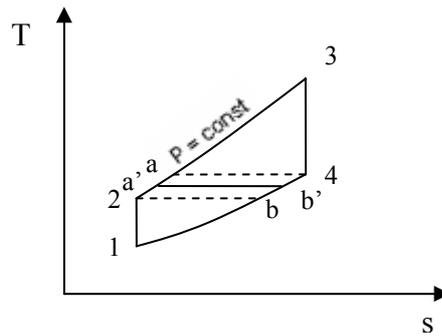
**Figure 3.3:** T-s Diagram for a regenerative GT cycle.
