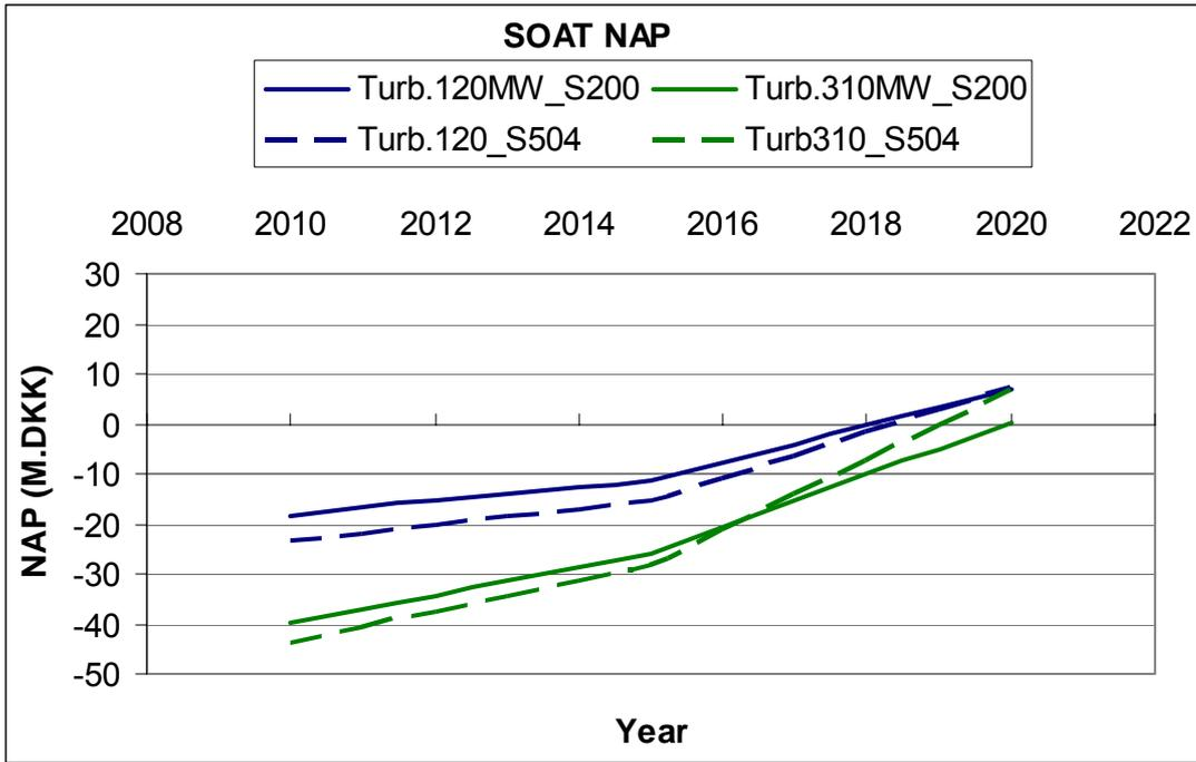
**Figure 5.8:** the Net Annual Profit (NAP) for the State of the Art Technology (SOAT) for two values of storage size (200,000 m<sup>3</sup> and 504,000 m<sup>3</sup>) and two turbine sizes (120 MW and 310 MW).
