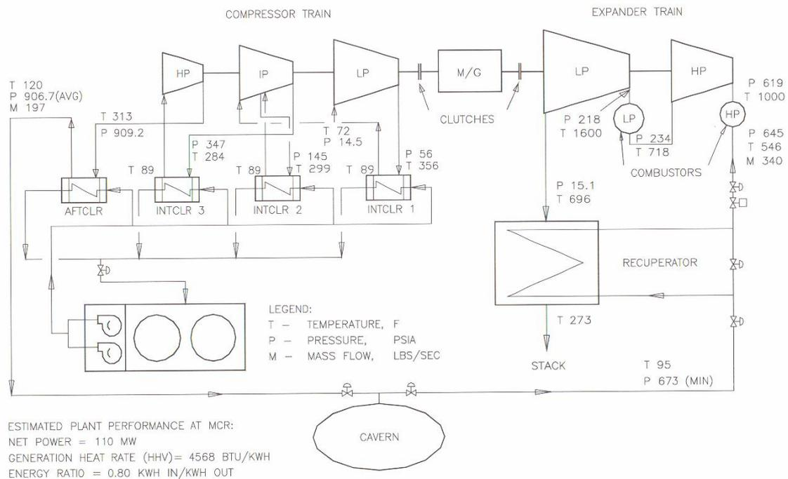
**Figure 3.9:** The Alabama plant schematic representation with main thermodynamic properties. Figure taken from (Boyce , 2002) where it is adopted from Energy Storage and Power Consultants, Inc. (ESPC) which has experience in “engineering, constructing, testing, and operating” the Alabama CAES plant.(www.espcinc.com)
