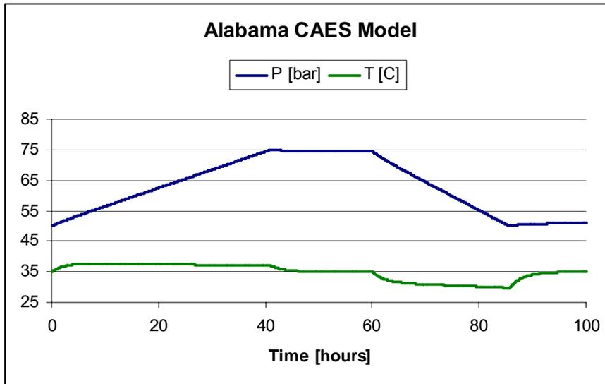
**Figure 4.2:** Model results for the variation of the storage temperature and pressure over an operational cycle.
