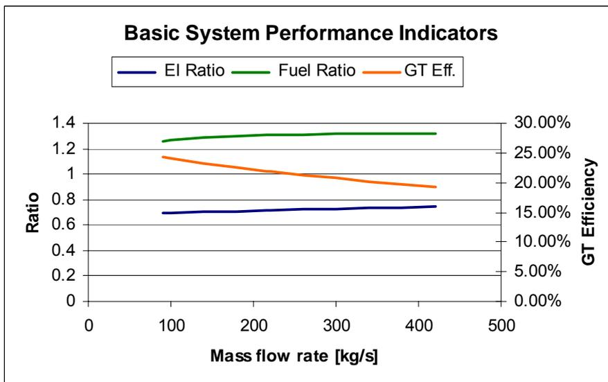
**Figure 4.3:** Basic system performance indicators for the CDT model at various turbine capacities, the main other capacities being the same as the Alabama plant.
