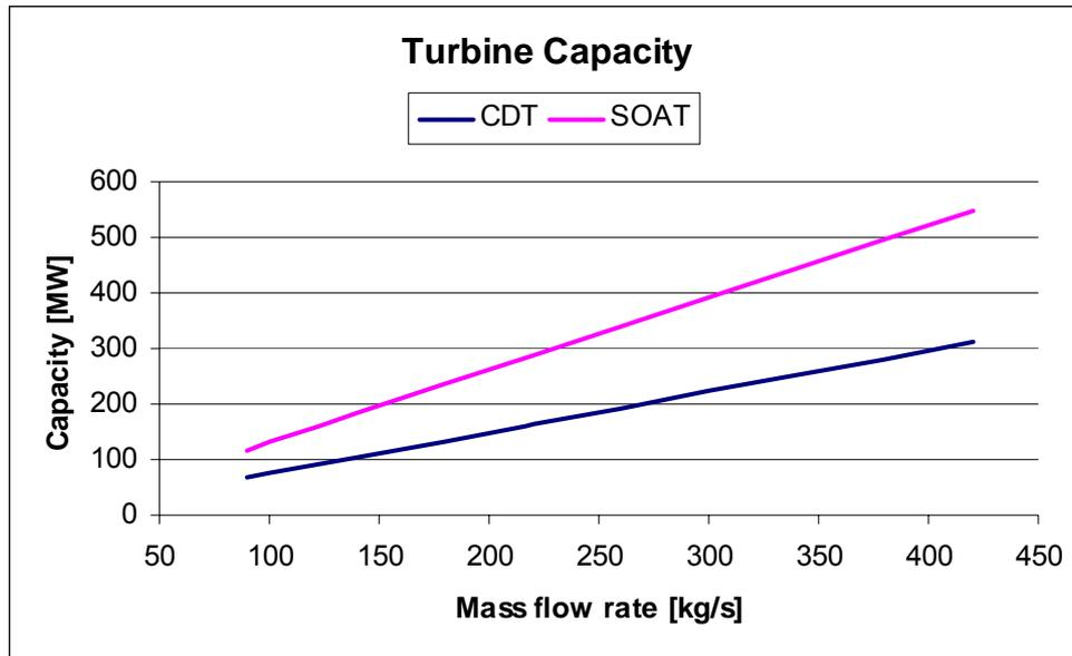
**Figure 5.1:** For the same air mass flow rate, turbines at higher firing temperature give a higher power output as shown by comparing the CDT and the SOAT results
