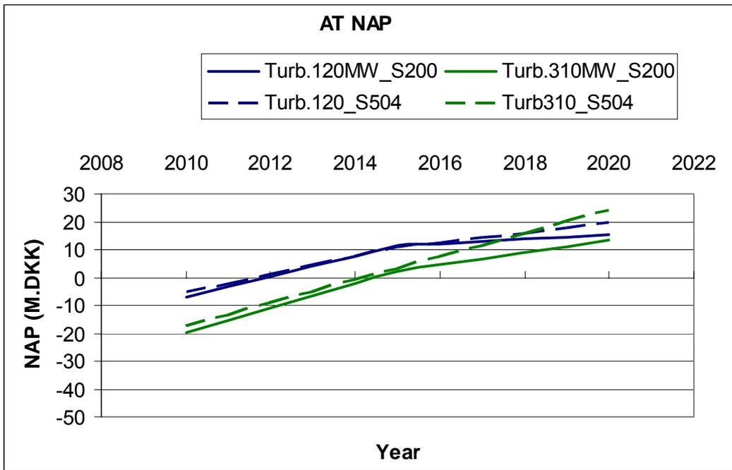
**Figure 5.9:** the Net Annual Profit (NAP) for the Current Day Technology (CDT) for two values of storage size (200,000 m<sup>3</sup> and 504,000 m<sup>3</sup>) and two turbine sizes (120 MW and 310 MW).
