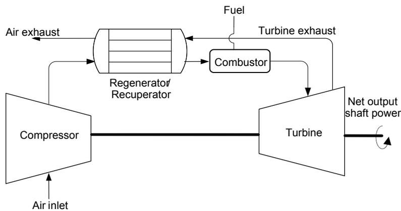
**Figure 3.4:** Schematic representation of a regenerative GT cycle.
