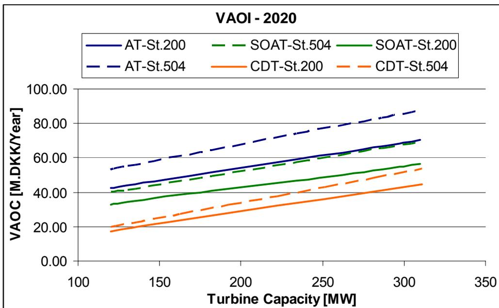
**Figure 5.5:** Variable Annual operational Cost (VAOI) for the year 2020 for various turbine capacities at cavern sizes of 200,000m<sup>3</sup> and 504,000m<sup>3</sup> respectively
