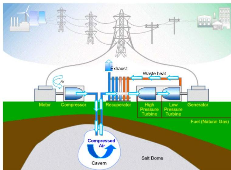
**Figure 1.1:** Basic CAES plant operation: air is compressed and stored in an underground cavern before being expanded in a gas turbine. (LCRA, 2003)
