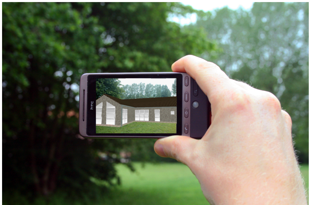
Figure 3.5: Photograph of HouseView in use. Using AR the virtual element is mapped to the surroundings using hardware sensors.
