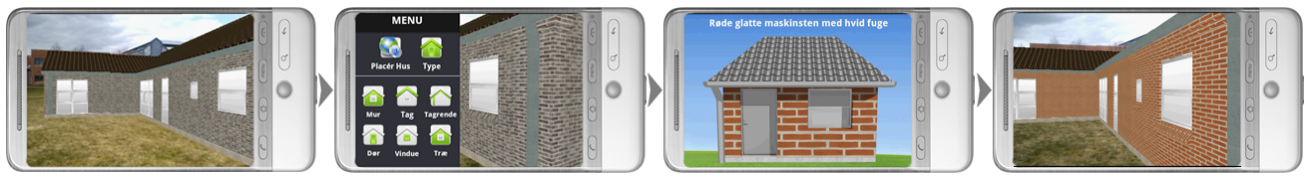
Figure 4. Series of screenshots showing the sequential process of changing materials. First image show a gray house. Second image shows the HouseView menu, with the gray house presented behind. Third image presents the Material View, where it is possible to scroll a series of different materials. Last image shows the same house, now build with the red brick selected in the Material View.
