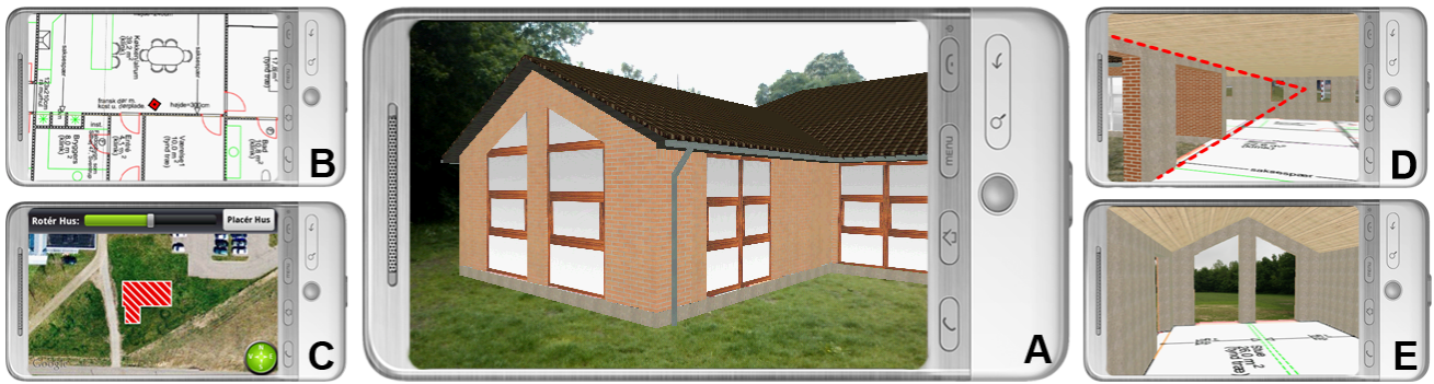
Figure 2. User interface of HouseView - A: Screen capture of a virtual house positioned on a lawn. B: Screen capture of the Blueprint View, showing a general overview of the floor plan. The red square represents the user's position on the blueprint. C: Screen capture of the Placement View for house placement and rotation. The red shape represents the house, and the top bar makes it possible to rotate the house. D: Screen capture from inside the house. Notice the added dashed dividing lines between the roof and walls moving inwards and thereby creating perspective. E: Screen capture of the possible view from the living room. Notice how the real world is visible through the windows in the virtual walls.
