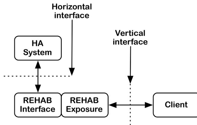
Figure 5.4: The interface orientations relevant to the interface and exposure of a home automation system through that interface.
