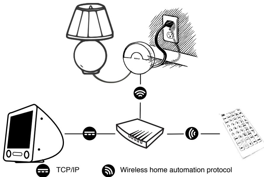
Figure 1.1: A typical home automation setup for controlling a lamp.
