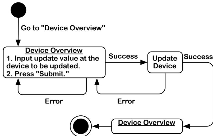
Figure 2.7: The state transitions involved in update a state attribute of a device. The “Device Overview” page can be replaced by a “Device Details” page without difference in state transitions.
