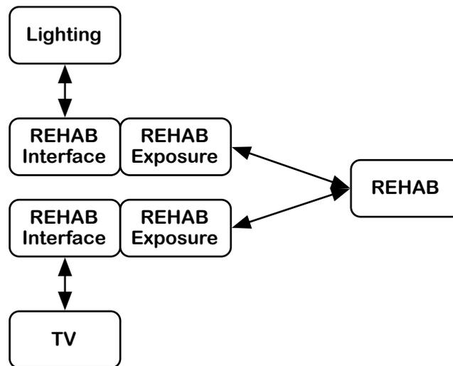
Figure 5.5: The communication to and from REHAB and home automation systems.
