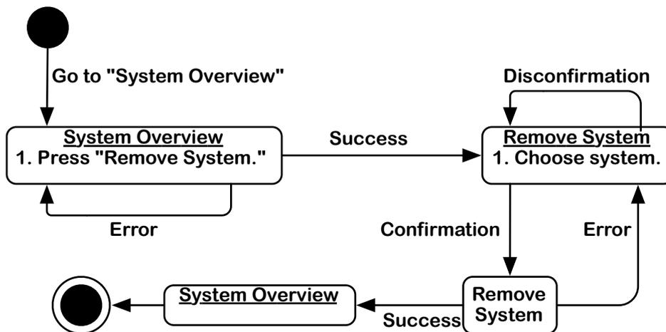
Figure 2.5: The state transitions relevant to removing a system from HAB.
