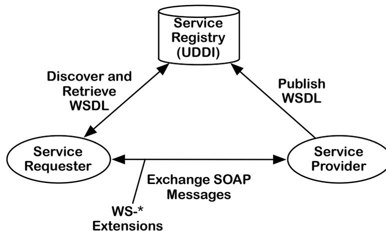
Figure 3.1: The basic principle of SOA.
