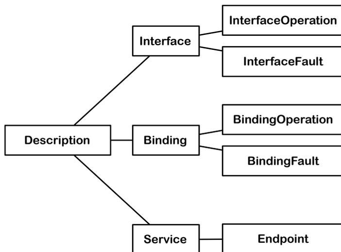
Figure 3.2: The WSDL 2.0 component model.
