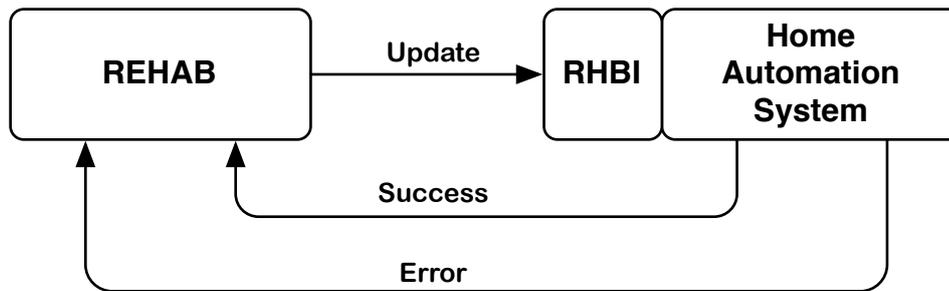
Figure 2.11: HAB issuing an update to a device, through the HAB interface (RHBI). The system containing the device report either success or failure in updating the device.
