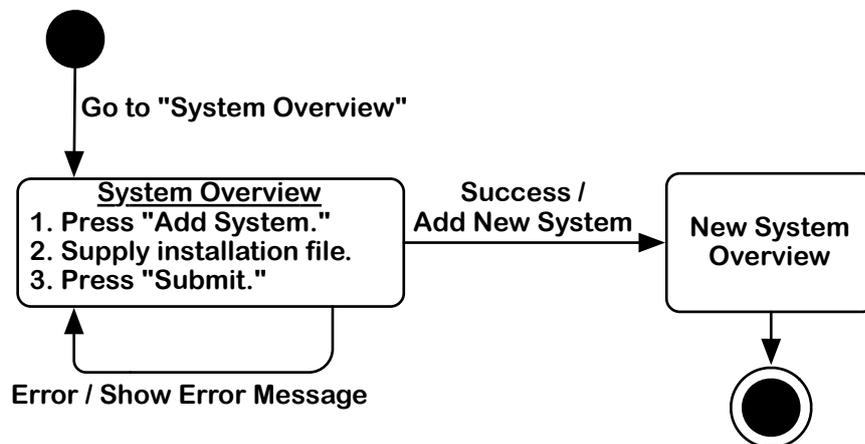
Figure 2.4: The state transitions when the Smiths want to add a new system to HAB.
