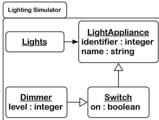
Figure 5.3: The model of the home automation lighting system.
