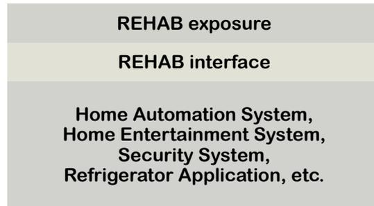
Figure 2.2: The HAB concept. The developer of the home automation related system in question implements the HAB interface that facilitates the exposure of domestic devices as Web services.
