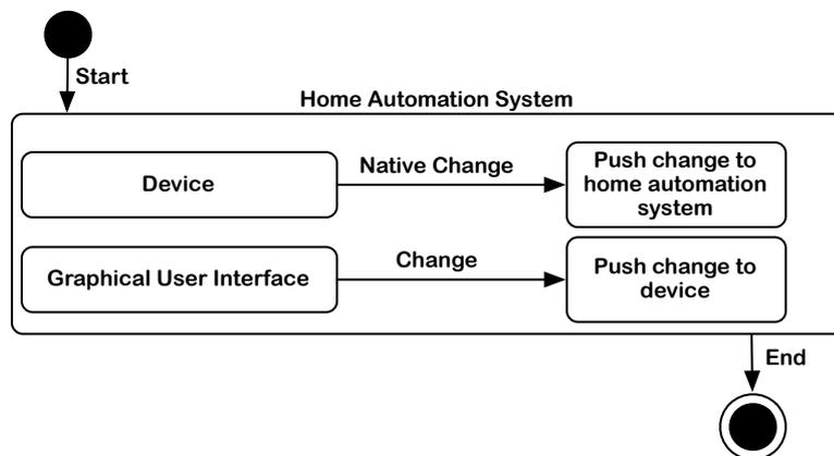
Figure 5.2: The behavioural model for a home automation system.
