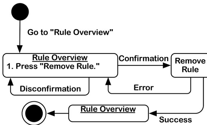
Figure 2.10: The state transitions involved in deleting a rule.
