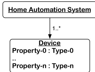
Figure 5.1: A general model for home automation systems. A system has a number of devices, which have a number of properties of varying type.
