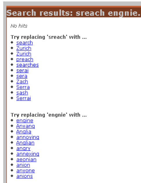
Figure 8.11 : If an empty result set is returned by KALCHAS the PHP script suggests alternative search terms
