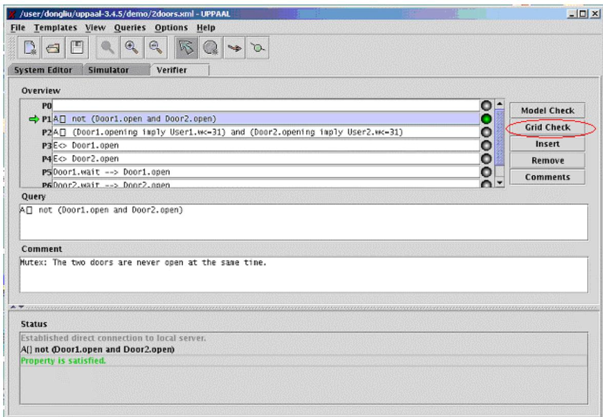
Figure IMP-04: “*Grid Check*” button in the Uppaal GUI
