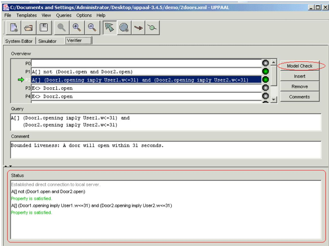
Figure IMP-01: The *SystemInspector* class starts the verification after users click the *Model Check* button.
