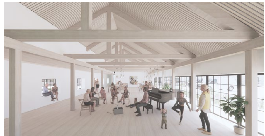
Illu. 177 - The gathering hall with an acoustic ceiling that decreases the reverberation times in the room to attain acoustic comfort.
