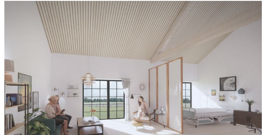
Illu. 175 - An apartment with an acoustic ceiling that decreases the reverberation times in the room to attain acoustic comfort.
