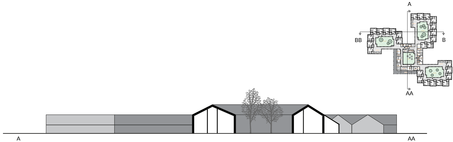
Illu. 85 - A-AA section in 1:500 that shows a difference in building height between the three residential departments and the common function department that connects them to create hierarchy in the building and enhance the communal areas.
