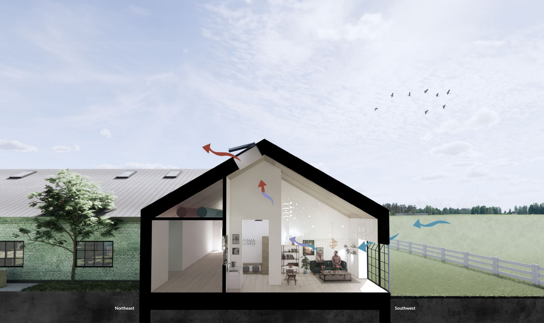
Illu. 166 - Section of an apartment that shows the natural ventilation principle based on thermal buoyancy, as well as the placement of the air supply inlet from the mechanical ventilation system in the wall above the living room.
