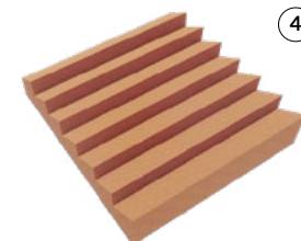
Illu. 119 - The shape of the acoustic ceiling panels. The influence on the ray behavior for each panel is examined in illu. 117-118 to the corresponding numbers.
