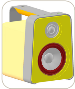
6. Front panel + Frame attached to the cabinet
