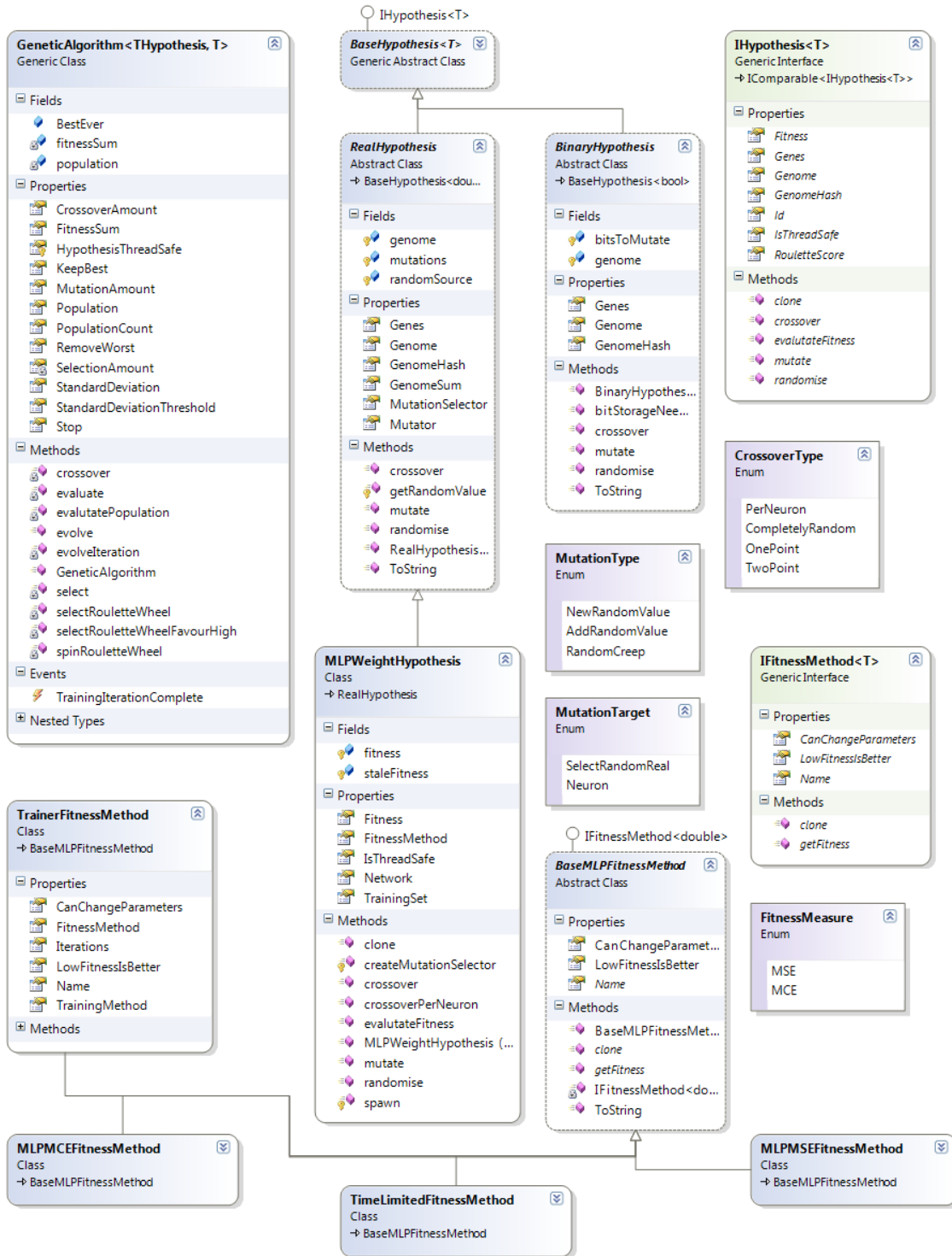
Figure 3.8: Classes used in the implementation of Genetic Algorithm for ANN weight training.
