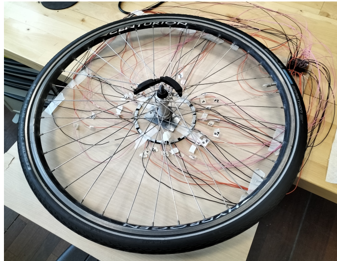
Figure 3.3: A picture of the horizontal wheel. The "crown" of hall effect switches can be observed, together with the multitude of wires connecting it to the ESP32 development board
