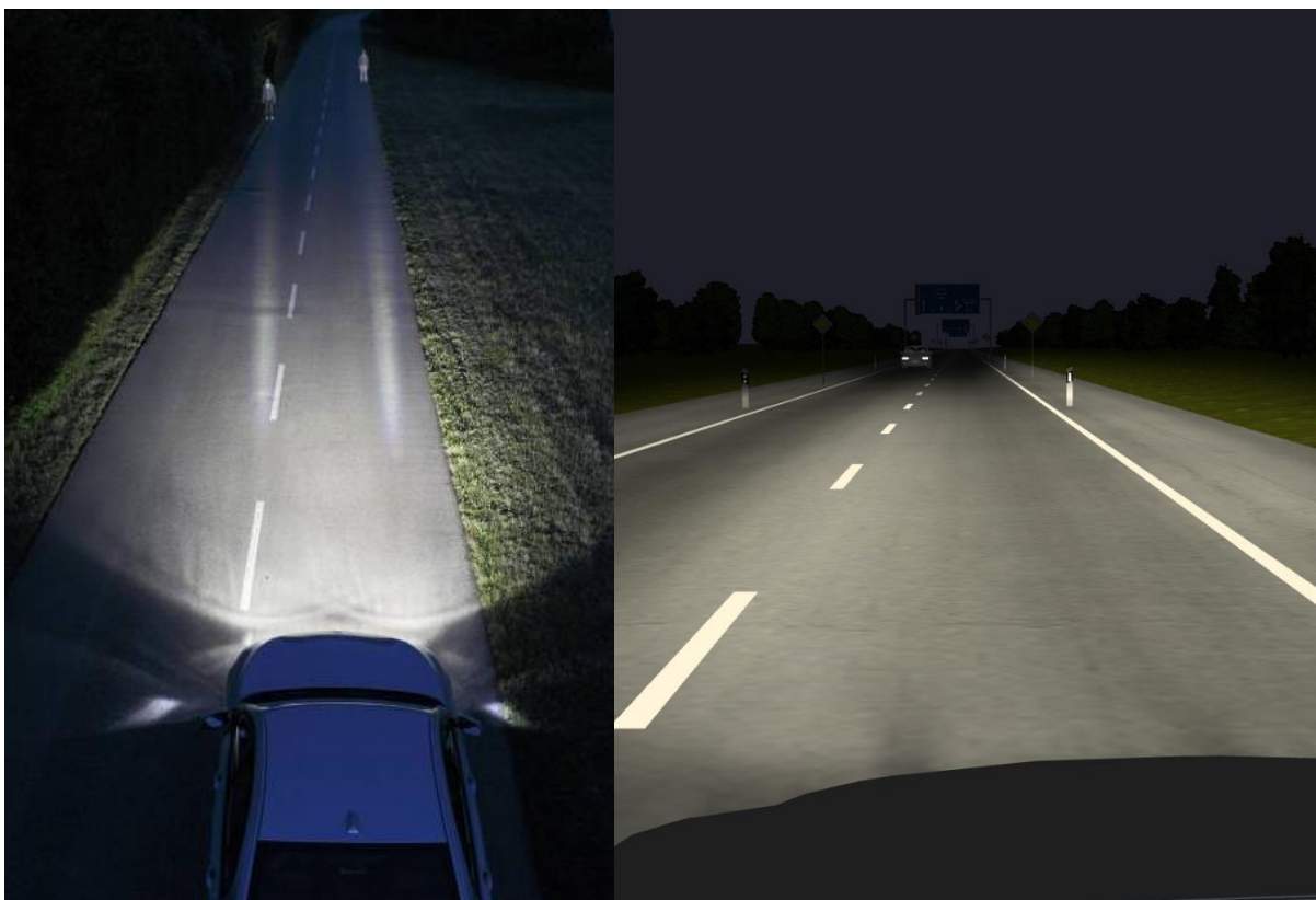
Image 17 On the left: Dynamic Light Spot. On the right: Glare-free high-beam assistant. BMW. 2011. ( Press.bmwgroup.com )
