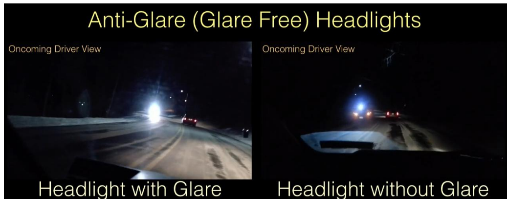
Image 21 Smart headlight, seen from the opposite driver's perspective. Carnegie Mellon. 2015. ( Cs.cmu.edu )
