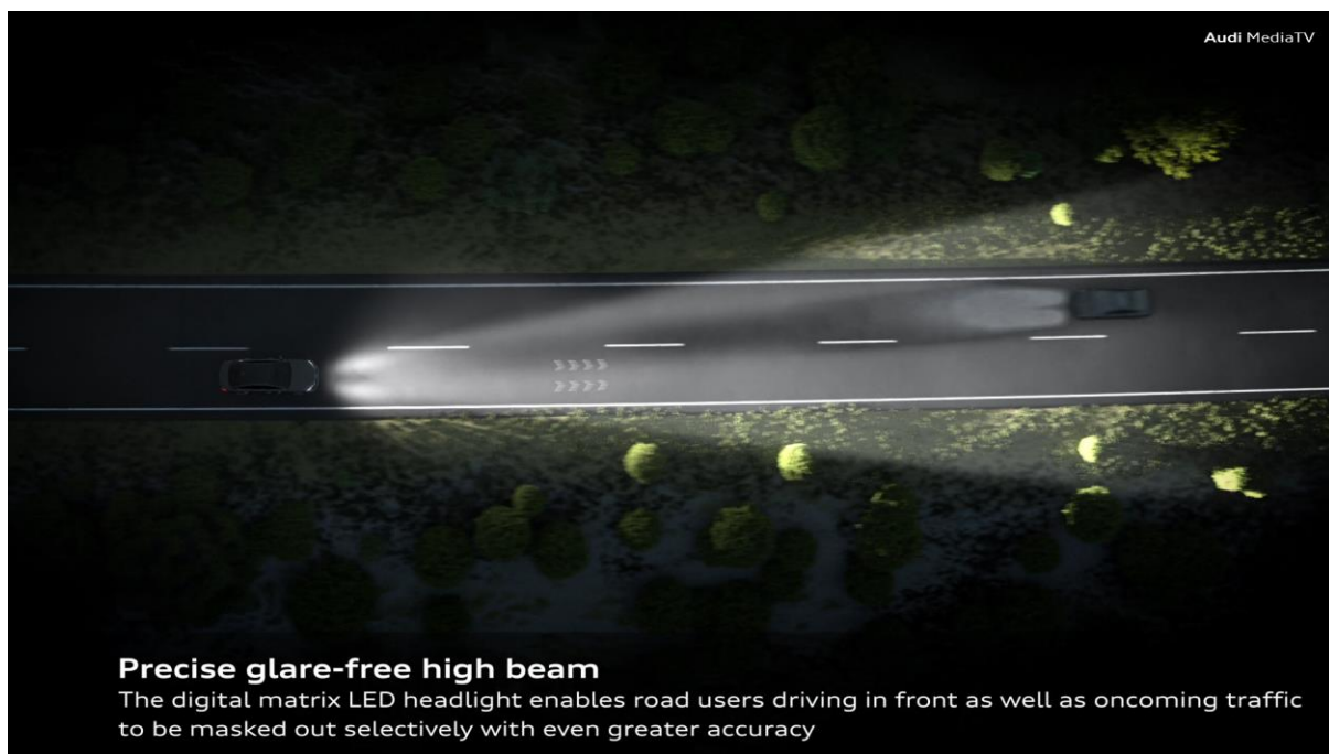
Image 20 Glare-free high beam. AUDI. 2022. ( Audi-mediacycenter.com )
