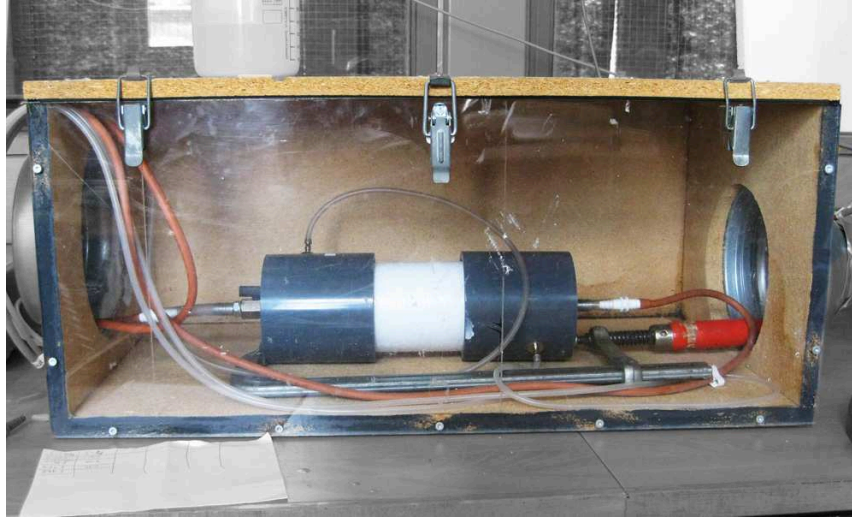
Figure 7.6: Pressure box with a specimen installed in the chambers
