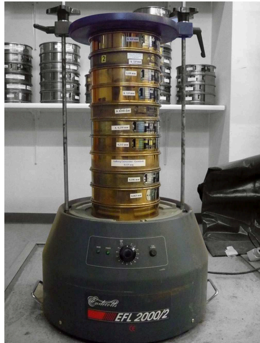
Figure 6.5: Set of sieves in the vibrating machine
