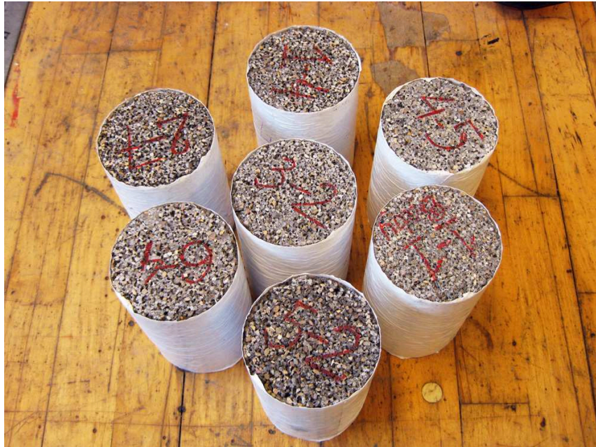
Figure 7.5: Set of specimens sealed with tape and ready for the test
