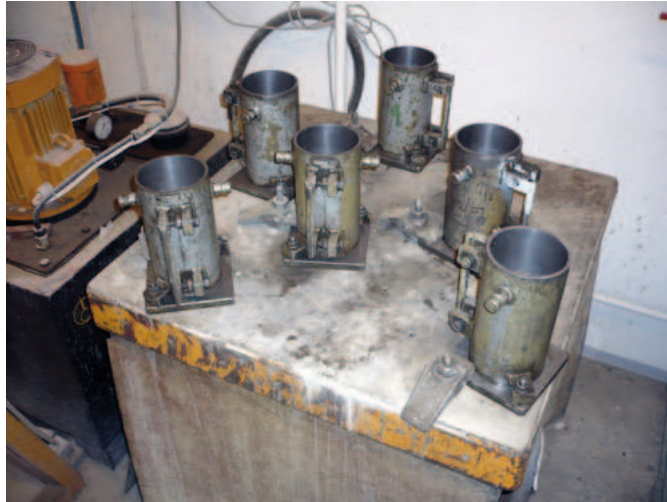
Figure 5.8: Vibration table with moulds bolted on it
