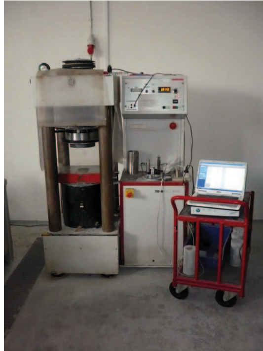
Figure 7.12: Tonipact 3000 compressive strength tester
