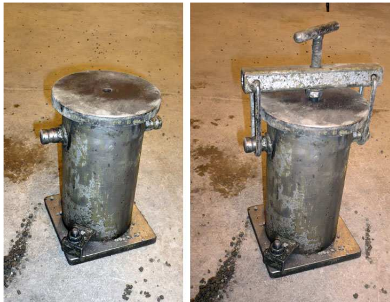
Figure 5.11: Clamping the mould
