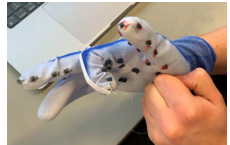
ill. 59. Band anchor points and test on distal phalange
