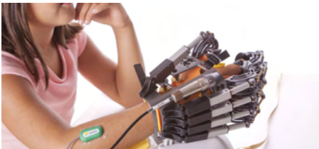
ill. 46. An exoskeleton glove with a very visible mechanical principle
