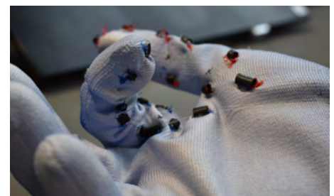
ill. 65. M. Abdelhafiz' cable routing on a glove
