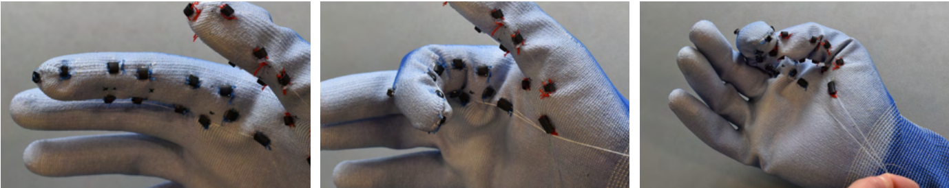
ill. 66. Simplified cable routing
