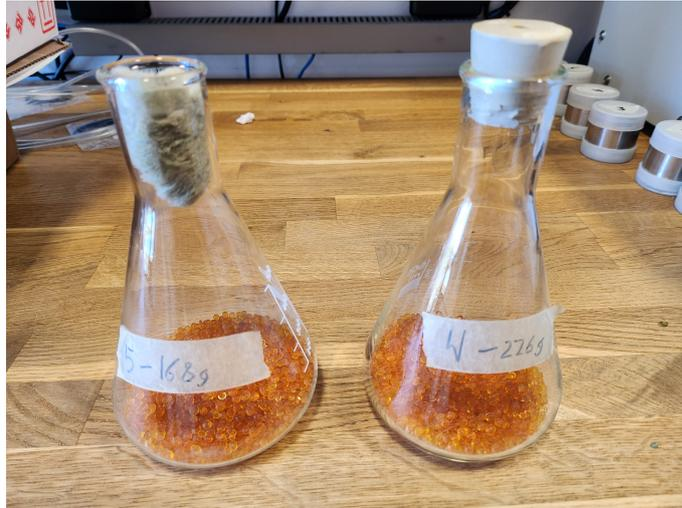
**Figure F.4** An example of two conical flasks, one with a RWI sample and one with a plug, to show the two different setups.
