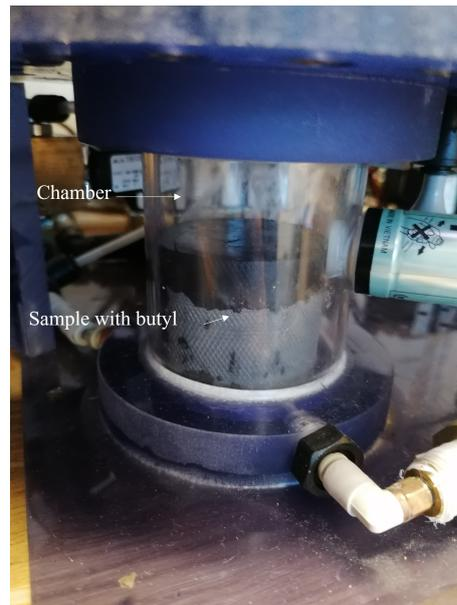
**Figure E.6** The chamber of a ODA20 with a plastic cylinder coated with Butyl.
