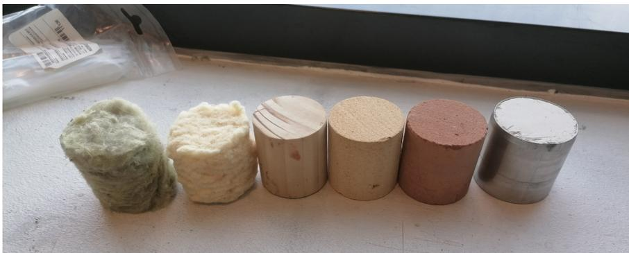
**Figure 0.1** A sample of each material used in this project. From left to right: Rockwool Insulation, Wood Fibre Insulation, Wood, Brick, Unfired Brick and Clay
