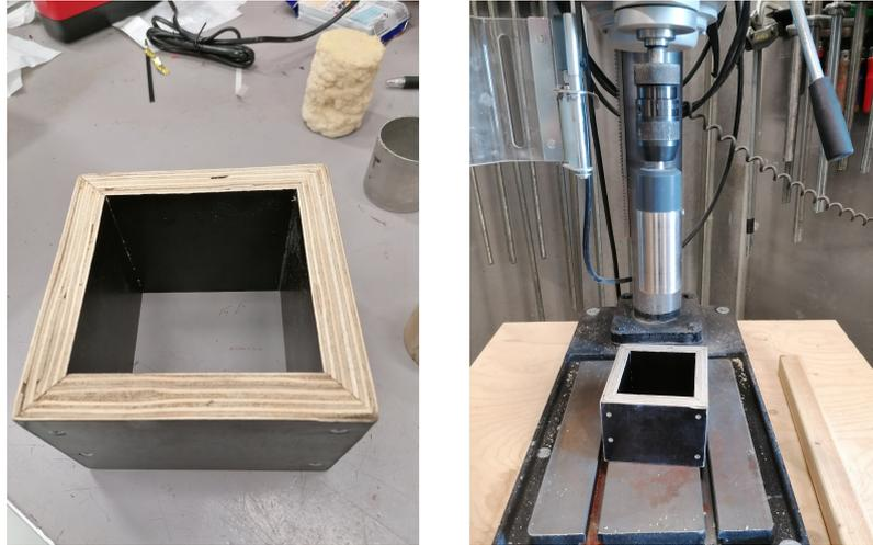
**Figure E.1** On the left: Wood frame with the inner dimensions of 95x95mm. On the right: The drill that cuts out the RWI sample with the wood frame placed under it.
