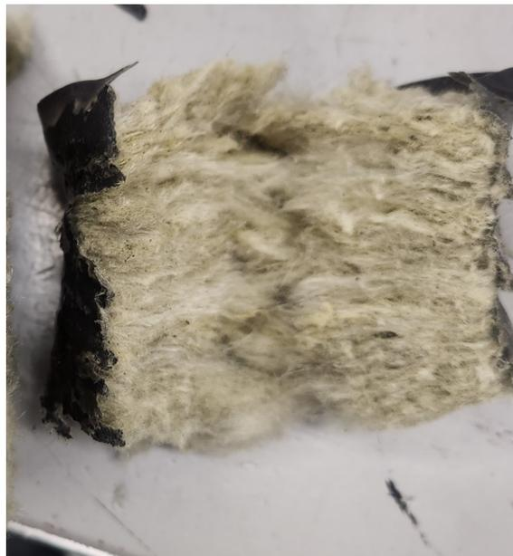
**Figure E.7** Cross-section of a RWI sample with MR on the sides. The MR does not penetrate the RWI.
