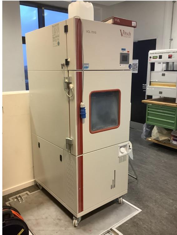
**Figure G.8** Picture of the VCL 7010 climate chamber.
