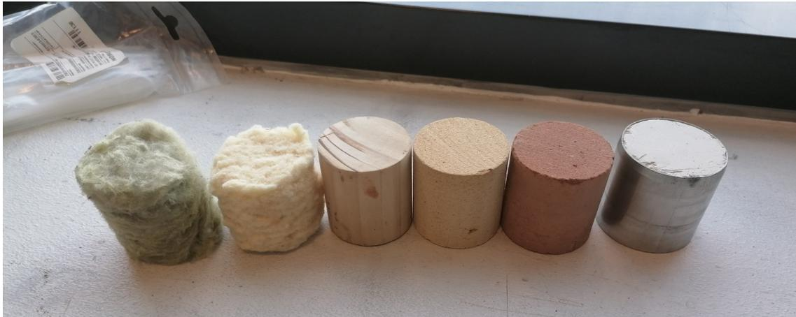
**Figure A.1** A sample of each material used in this project. From left to right: RWI, WFI, Wood, Brick, UBR and Clay.
