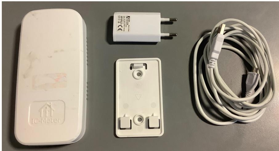
**Figure G.9** The IC-meter, the backplate, the power supply, and the cable.
