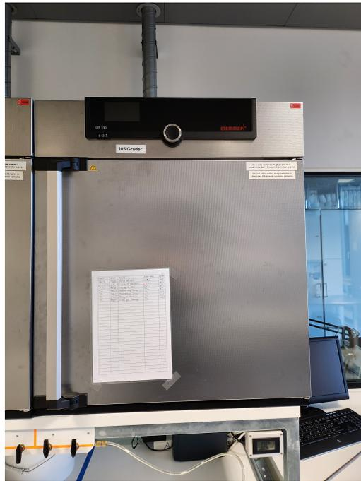
**Figure G.11** The Memmert UF110 heating oven used for the silica gel. The oven has the internal dimensions of 560 x 480 x 400 mm and is sat to 105 °C.
