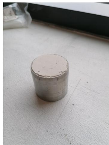
**Figure E.15** A clay sample packed in a metal cylinder.
