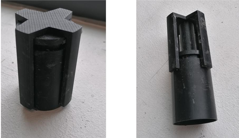
**Figure G.4** A device to push down the soft materials. This will ensure that the samples are not compressed. On the left; device when the stamper is down. On the right; when the stamper is up.
