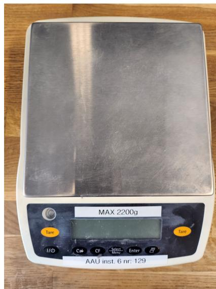
**Figure G.1** Picture of ENTRIS 2202 1S with the dimensions, D x W x H, 230 x 303 x 91 mm. [60]
