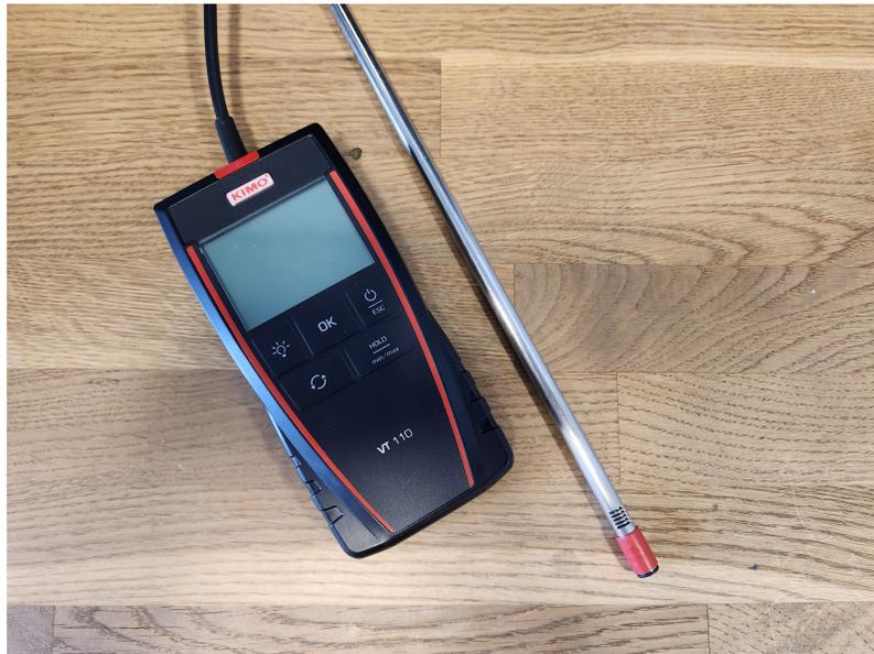
**Figure G.15** The Kimo VT110 Anemometer used for the air velocity in the climate chamber.
