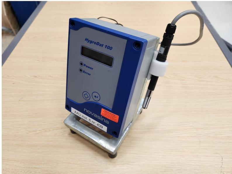
**Figure G.14** Novasina Hygrodat 100 Precision humidity Sensor used for the quality control of RH.
