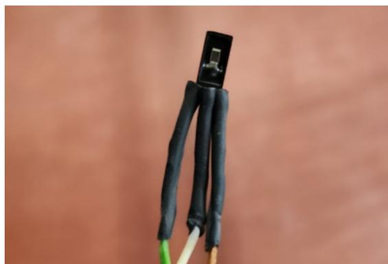
**Figure G.12** The Honeywell humidity sensor used for the silica gel experiments.
