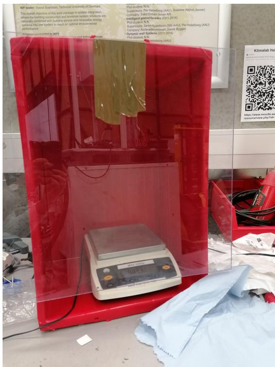
**Figure G.2** Setup with the balance in a box with Plexiglas.
