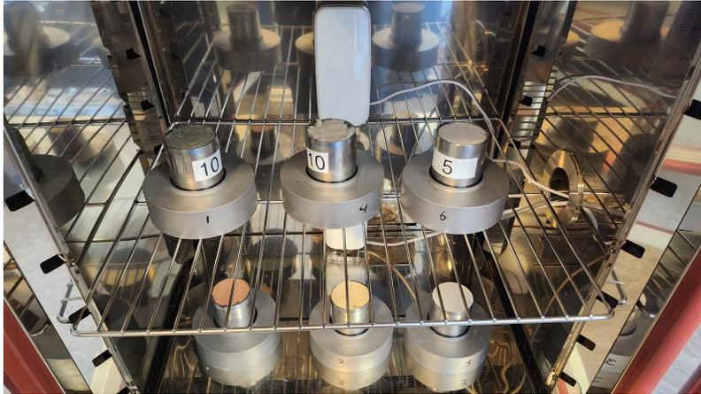
**Figure C.5** The picture showcases the interior of a climate chamber, where the six test assemblies can be seen.
