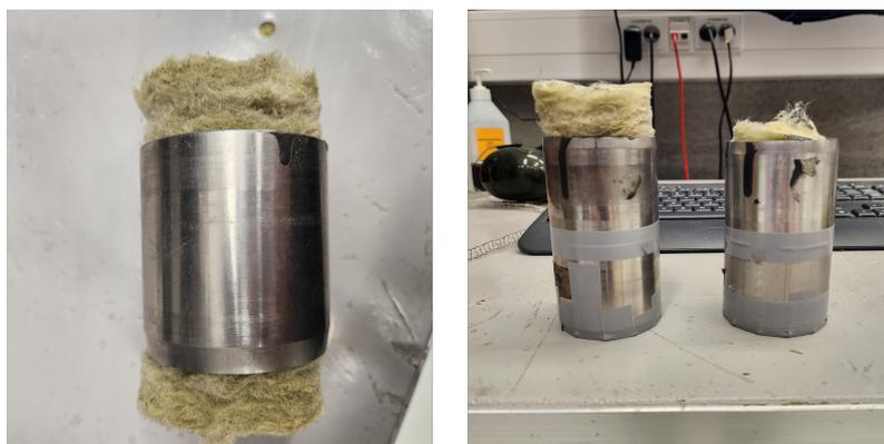
**Figure E.12** On the left: A RWI sample cut a little longer than the cylinder. On the right: A RWI sample that is placed into the cylinder. Underneath another cylinder to capture the rest of the MR.
