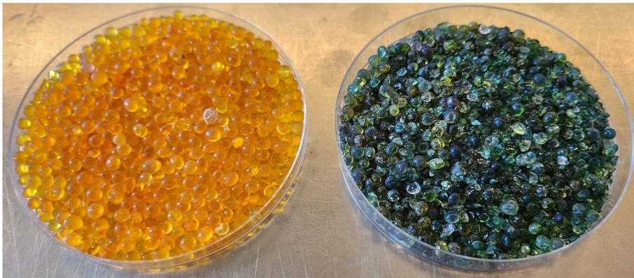
**Figure F.2** A picture of orange silica gel. As the silica gel adsorbs moisture, its color change from orange color to green, indicating that it has reached its maximum capacity for moisture adsorption.
