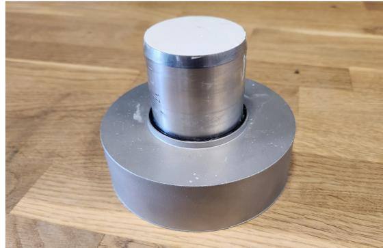
**Figure C.1** 3D model of the test assembly showing the cylinder, O-ring, and test cup. **Figure C.2** A picture of a example of a test test assembly used in the experiments.
