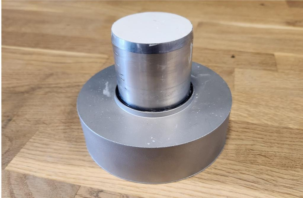
**Figure H.9** A picture of the final SLS printed test cup with a test sample installed.
