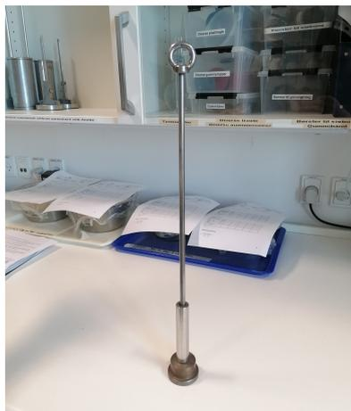
**Figure E.14** Stamper for stamping the clay into the cylinder.
