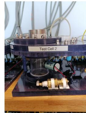
**Figure 0.4** The ODA20 and a test sample.
