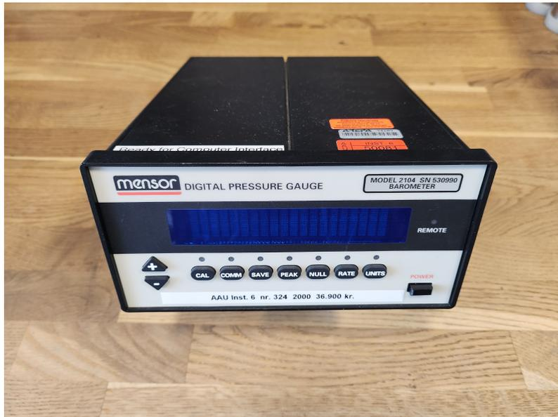
**Figure G.10** The Mensor 2104 digital pressure gauge.
