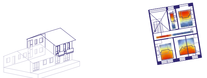
(III. 182) Iteration 08. Daylight provision on 1st floor of single and 2-storey houses.
