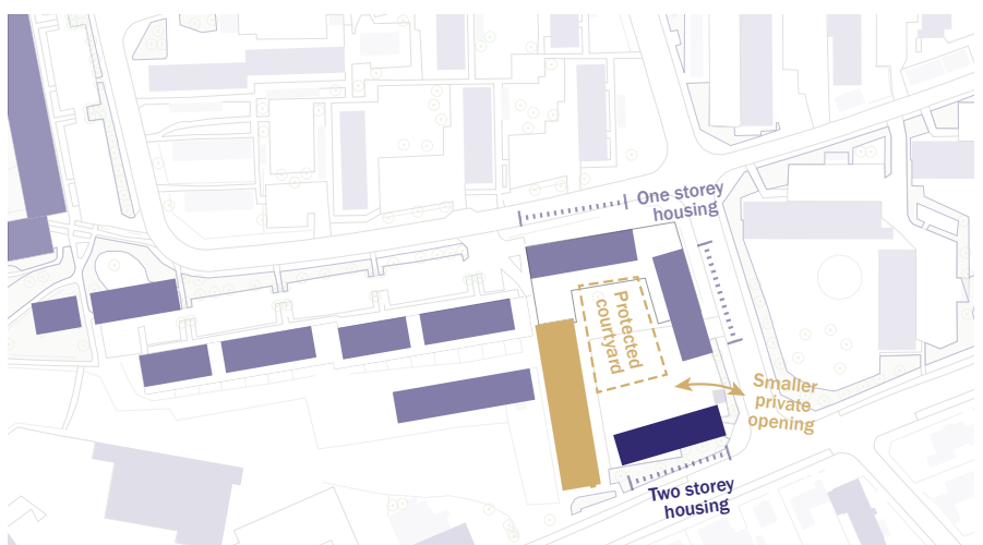
III.124 | Proposal to isolate the area from Sundvej's traffic noise on the south.
