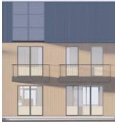
(III. 222) Wooden facade facing south with solar panels in a two-storey house. 1:200
