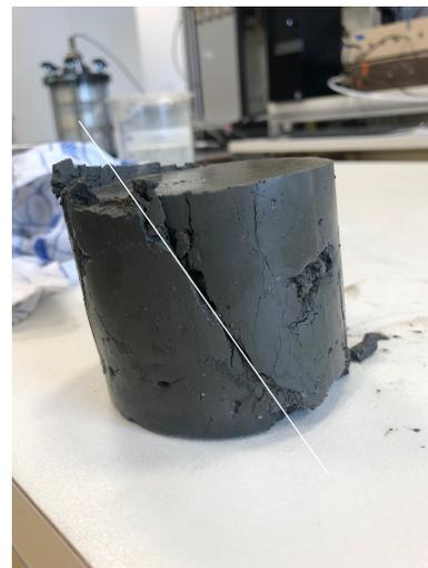
(b) Shear band failure mechanism.
