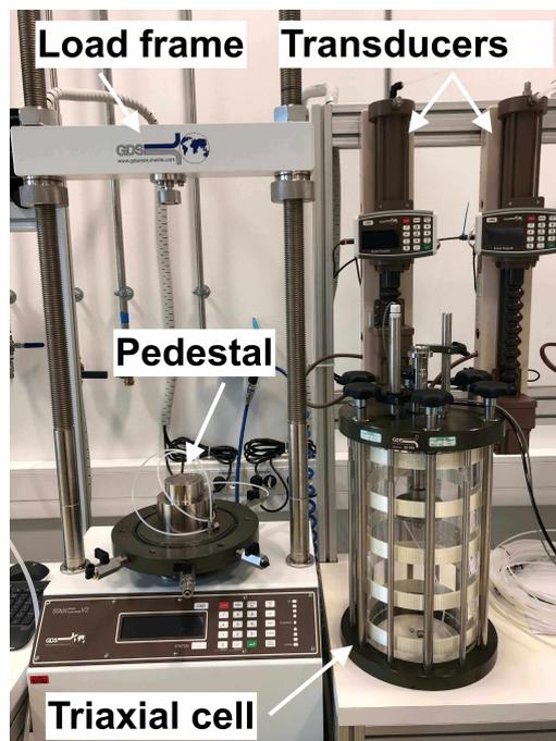
*Figure C.1.* GDS Triaxial Automated System (GDSTAS) setup.
