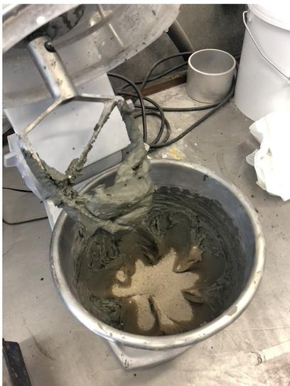
(a) Adding cement to the remolded soil.
