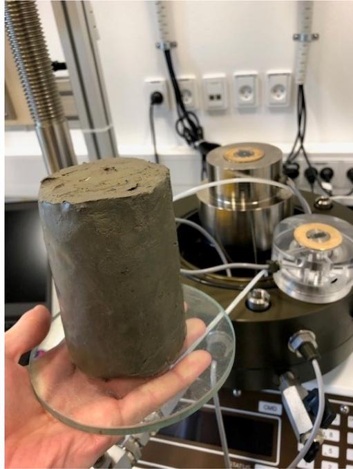
*Figure C.4.* GDS Bender Element System (GDSBES) setup in GDSTAS.
