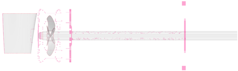
Figure A.20: Mesh visualisation of the cell quality below the values of 0.3.
