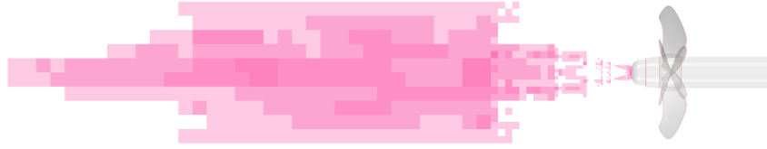
Figure A.5: Mesh visualisation of intermittency residual below the values of -1.0 \cdot 10^{-5} and above 1.0 \cdot 10^{-5} .
