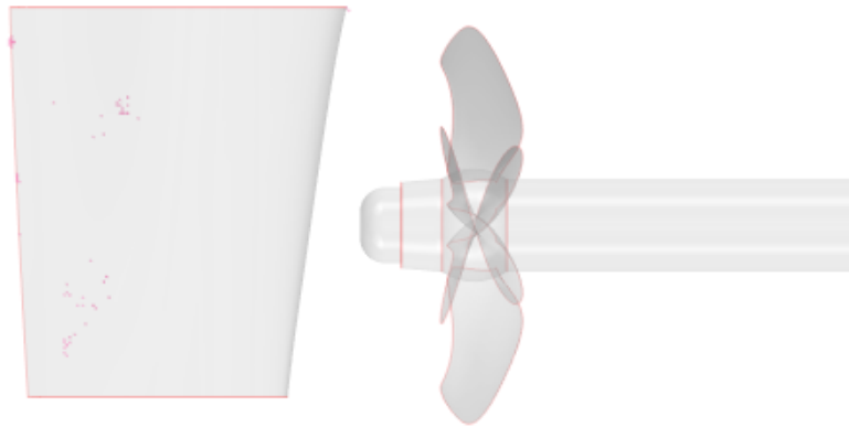
Figure A.22: Mesh visualisation of mass imbalance (continuity) residual below the values of -1.0 \cdot 10^{-6} and above 1.0 \cdot 10^{-6} .
