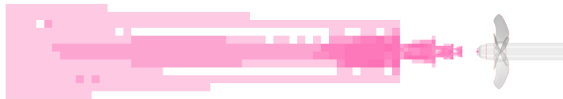
Figure A.7: Mesh visualisation of X-, Y- and Z-momentum residuals below the values of -1.0 \cdot 10^{-5} and above 1.0 \cdot 10^{-5} .
