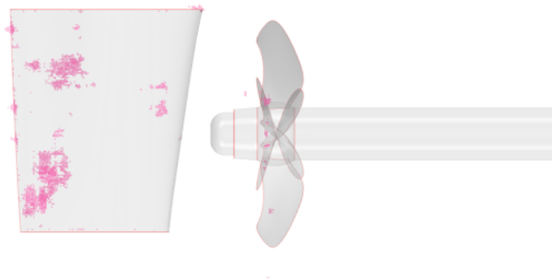
Figure A.24: Mesh visualisation of the specific dissipation rate below the values of -0.01 and above 0.01 .
