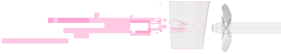
Figure A.21: Mesh visualisation of intermittency residual below the values of -1.0 \cdot 10^{-5} and above 1.0 \cdot 10^{-5} .
