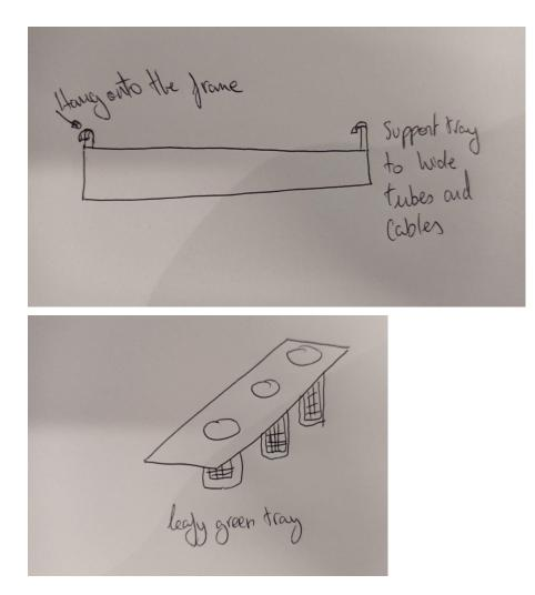
With these designs in mind, the next step is taken. This step consists of putting the draining tray on top of the support tray.
