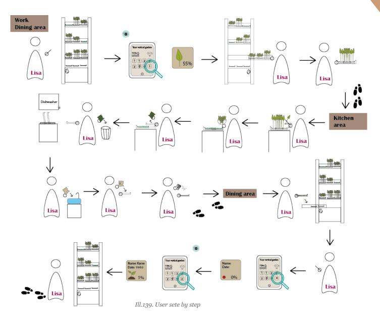
In the morning, the user checks the app to see what is ready to be harvested. Then they harvest and place the growing medium in the bin. The tray then goes into the dishwasher and the user has to prepare a new tray with seeds. This tray then does into the germination drawer and after three days it is put on the watering system.
