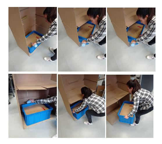
Arter the positioning of the opening was decided (Front), some parameters where set. It needed to be discrete, easy to open and it needed to be closed, so water would not evaporate. Due to this different water caps where tested out.
