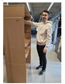
*Ill.96. Testing out the accesibility to highest shelf when 7cm has been added for 6 layers*
