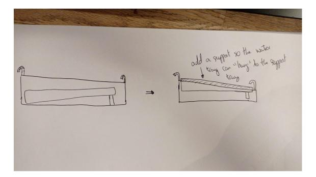
As can be seen on the left-hand side of the picture, the draining tray could easily just sit at the bottom of the support tray. In this case, the outlet of the tray would tilt it in the wrong direction completely negating the effect of the incline. Because of this, a support rim is added to the draining tray so it can sit on the edges of the support tray.
