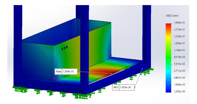
Ill.135. FEA maximum deformation simulation water tank
