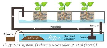
The nutrient film technique consists of prividing a thin layer of nutrient solution to the roots of the plants. Unlike the deep water culture, the plants are not always submerged in water. These are suspended on an inlcine surface so that the solution recirculate back into the water tank. [Bulla, A. (2022)]
