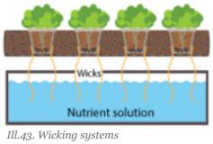
Represents the simplest form of hydroponic systems, requiring no water or air pumps. In these systems, the wick absorbs the nutrient-rich water and provides it to the plants. This system does not work well for large greens. It is also not considered to be a good solution for vertical gardens. [Bulla, A. (2022)]
