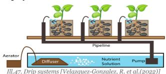
In this system, all plants are watered individually through a pipeline system. A timer is used to water the plants. Because of the the amount of pipes and hoses, leakage is common [Bulla, A. (2022)]. Probably not a good fit for restaurant use.
