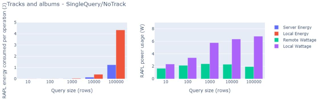
Figure 3.9: The energy efficiency of the Tracks and Albums query and NoTracking/Single query setting.
