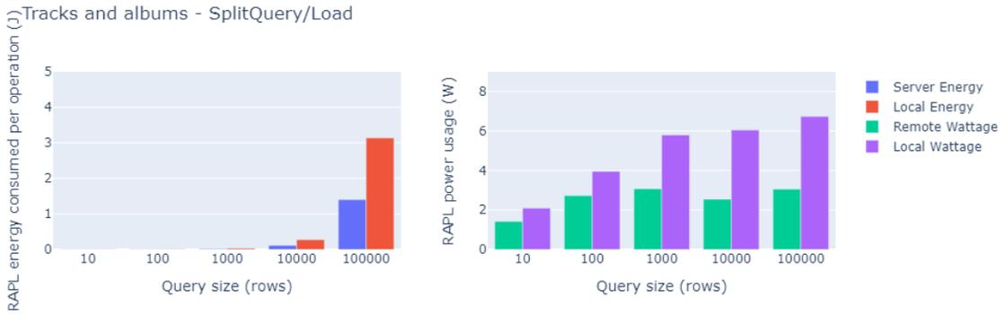
Figure 3.13: The energy efficiency of the Tracks and Albums query and Load/Split query setting.
