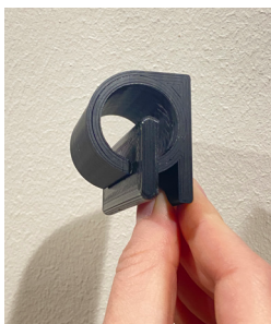
ill. 112 3d printed rotation hinge
