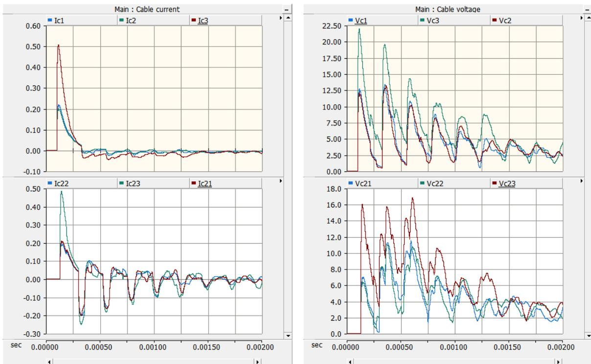
Figure 6:6 Overvoltage and current in cable: Lightning | Shield wire; Grounding Configuration | 'separate points'; Sheath | cross bonded
