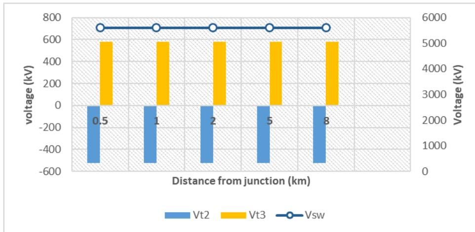
Figure 6:16 Impact of grounding location on OHL
