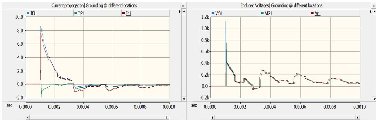
Figure 7:1 Current propagation and induced voltages during lightning strike on phase conductor
