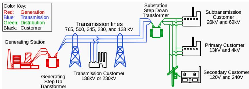
Figure 1:1 : Electrical Power System [3]
