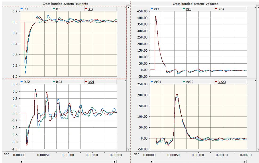
Figure 6:4 Overvoltage and current in cable: Lightning|Shield wire; Grounding Configuration|Short circuit; Sheath|cross bonded
