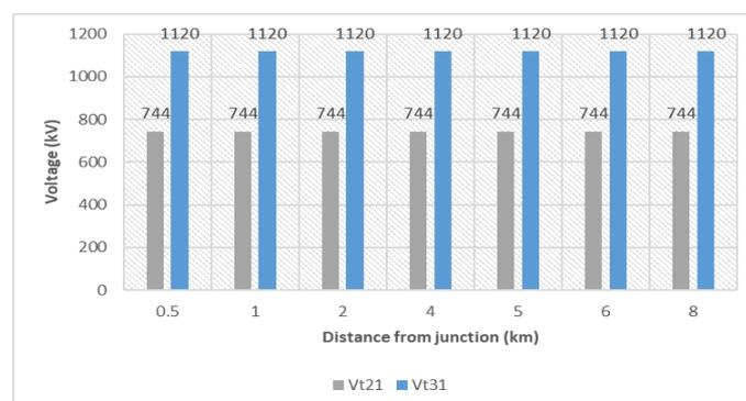
Figure 7:9 Impact of grounding location distance on OHL induced voltages: Lightning | Phase conductor
