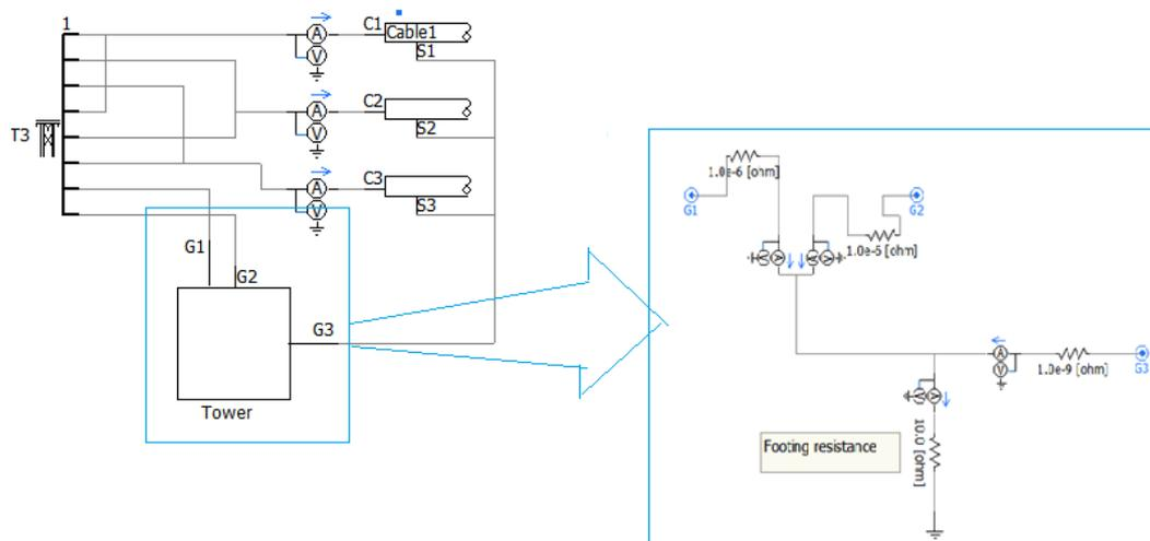
Figure 3:1 Grounding configuration 'A': 'short circuit'
