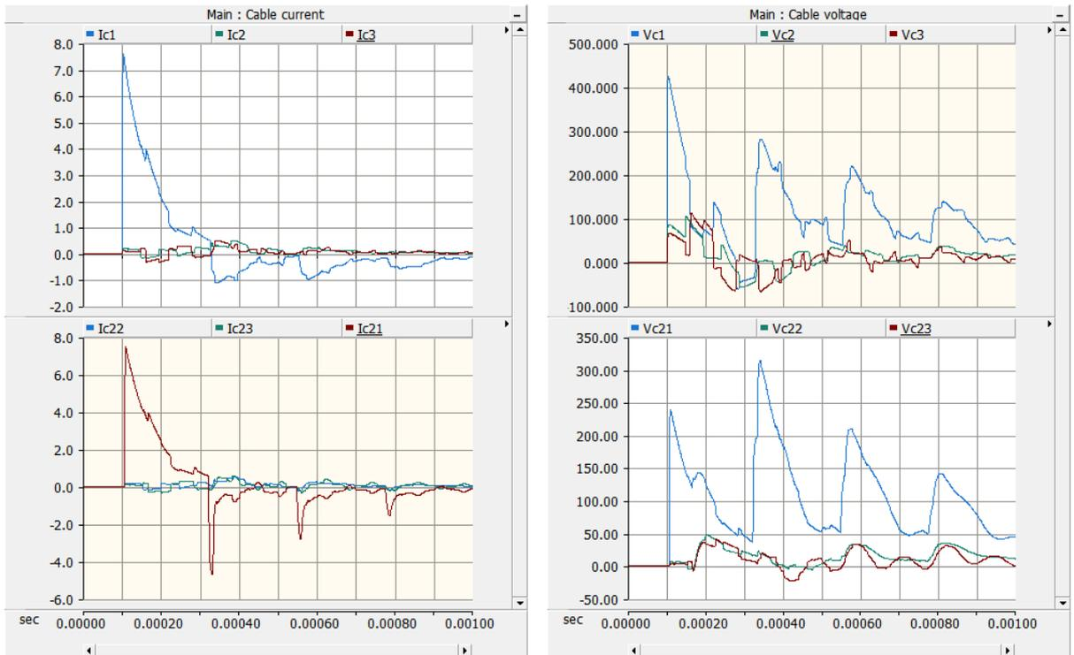
Figure 7:4 Overvoltage and current in cable: Lightning| Phase conductor; Grounding Configuration | 'different locations'
