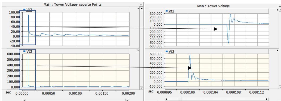
Figure 6:11 Upper phase voltage at Tower 2 and 3 for different grounding methods when lightning strikes shield wire. Grounding method| ‘separate point’
