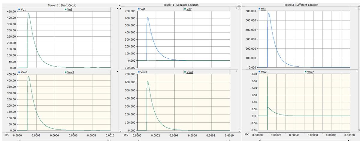
Figure 6:2 Induced over voltages in shield wire and cable sheath
