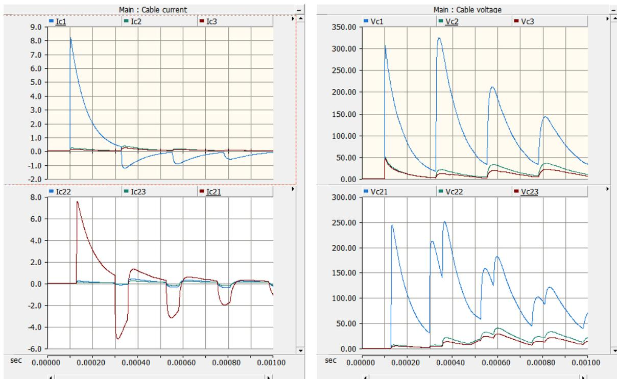
Figure 7:2 Overvoltage and current in cable: Lightning | Phase conductor; Grounding Configuration | Short circuit
