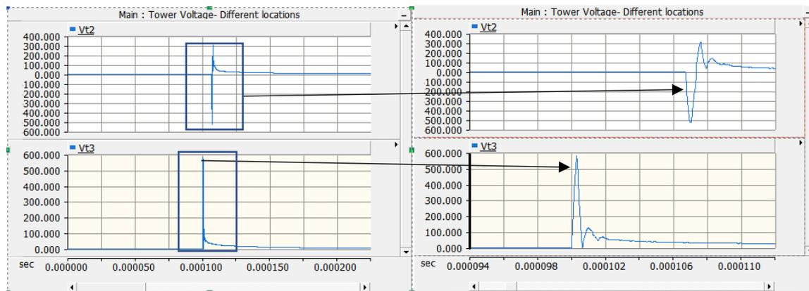
Figure 6:12 Upper phase voltage at Tower 2 and 3 for different grounding methods when lightning strikes shield wire
