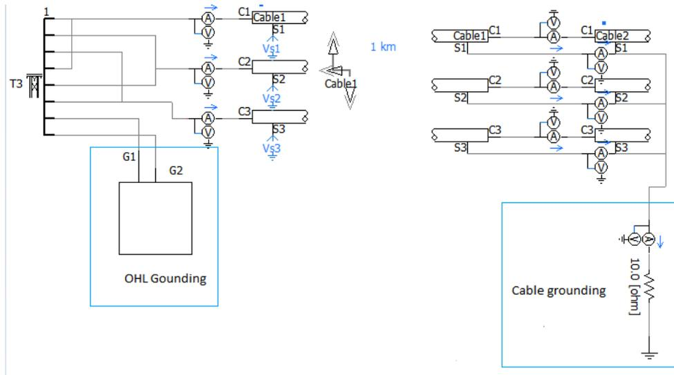
Figure 3:3 Grounding configuration 'C': 'different locations'
