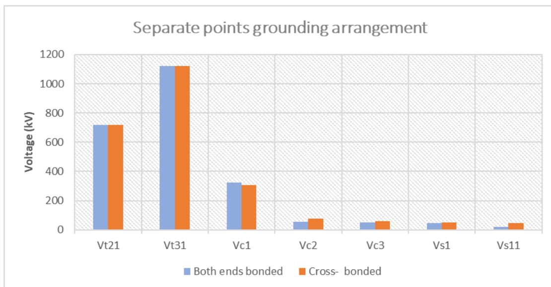
Figure 7:13 Impact of cross-bonding: Grounding method| 'separate point' s, Lightning| Phase conductor
