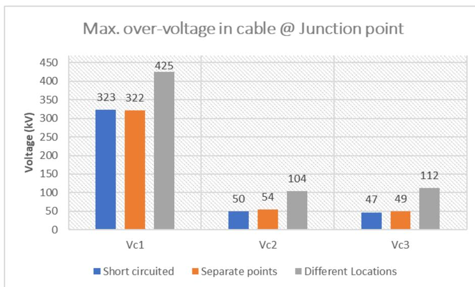
Figure 7:6 Comparison of maximum phase over voltage in cable at the junction point: Lightning| Phase conductor
