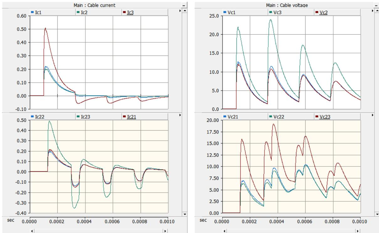
Figure 6:5 Overvoltage and current in cable: Lightning | Shield wire; Grounding Configuration | 'separate points' ; Sheath | Both end bonded
