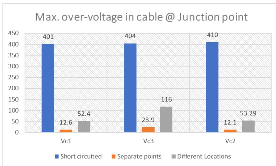
Figure 6:13 Comparison of maximum phase over voltage in cable at the junction point:
