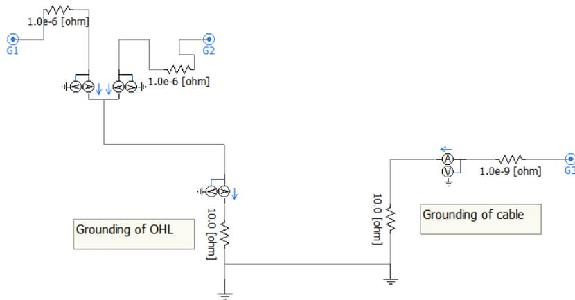
Figure 3:2 Grounding configuration 'B': 'separate points'
