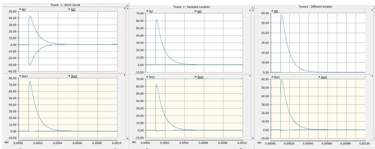
Figure 6:1 Current in Shield wire and Sheath in case of fault on Shield wire
