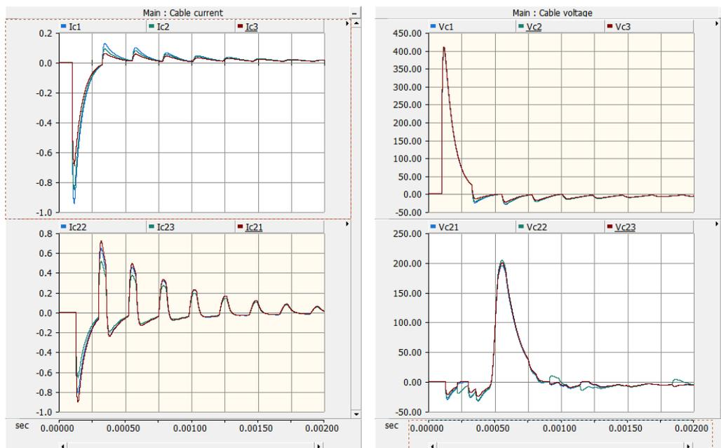
Figure 6:3 Overtoltage and current in cable: Lightning|Shield wire; Grounding Configuration|Short circuit; Sheath|both-end bonded
