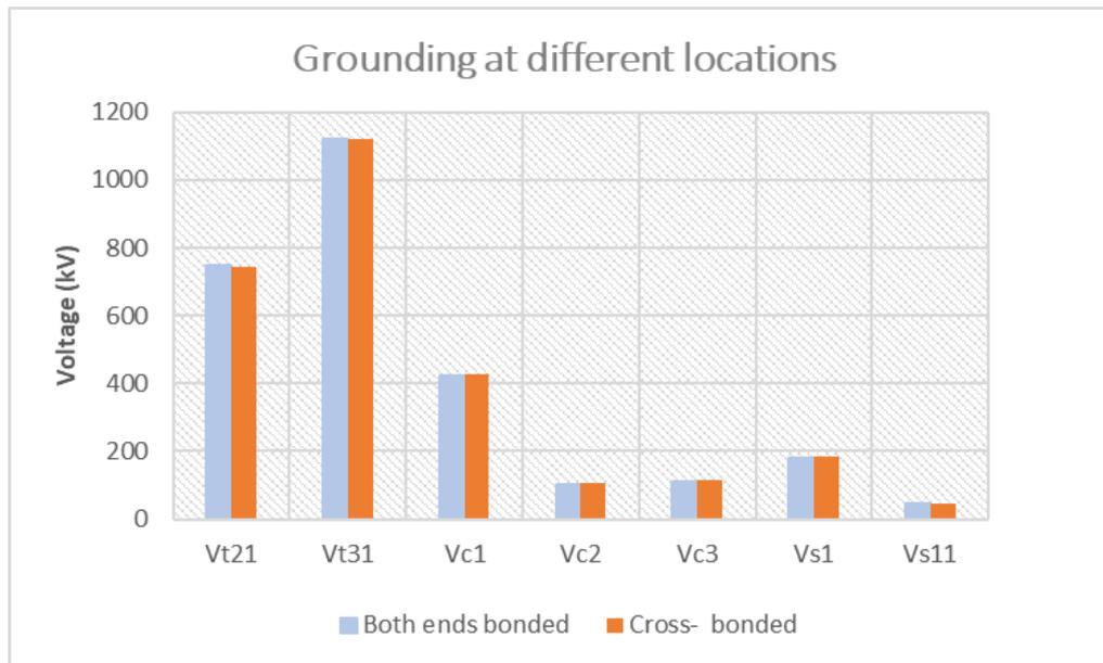
Figure 7:14 Impact of cross-bonding: Grounding method | 'different location' s, Lightning | Phase conductor
