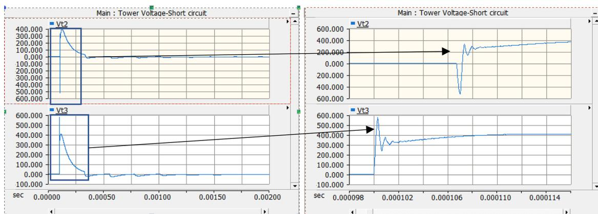
Figure 6:10 Upper phase voltage at Tower 2 and 3 for different grounding methods when lightning strikes shield wire. Grounding method| Short circuit
