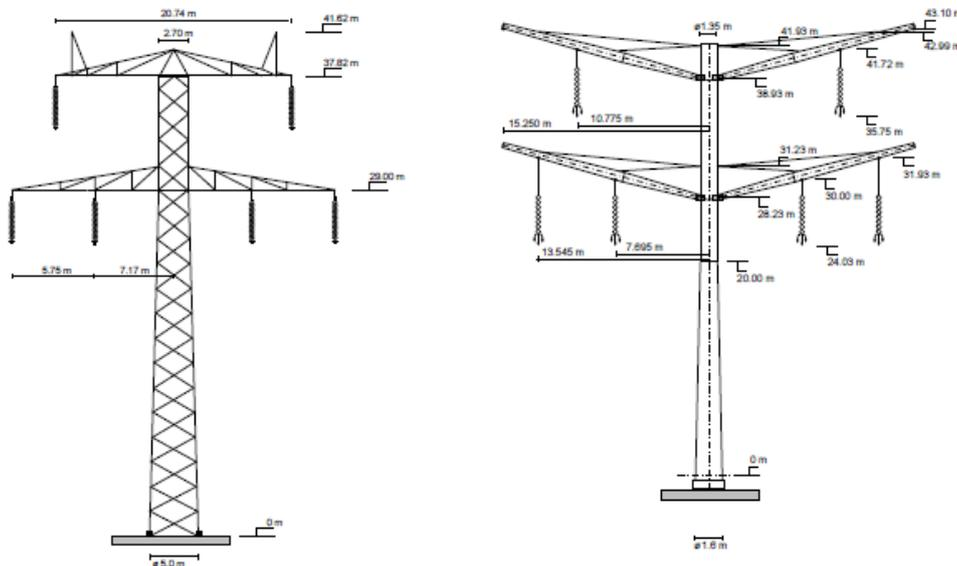
Figure 1:3 : Donau Pylon on the left and Eagle Pylon on the right [9]
