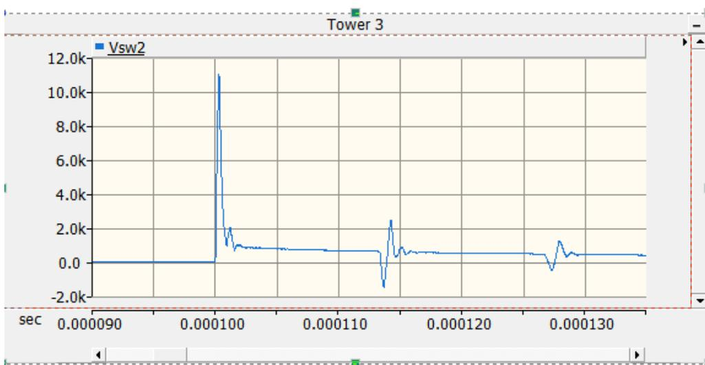
Figure 6:15 Voltage in Shield wire when lightning strikes
