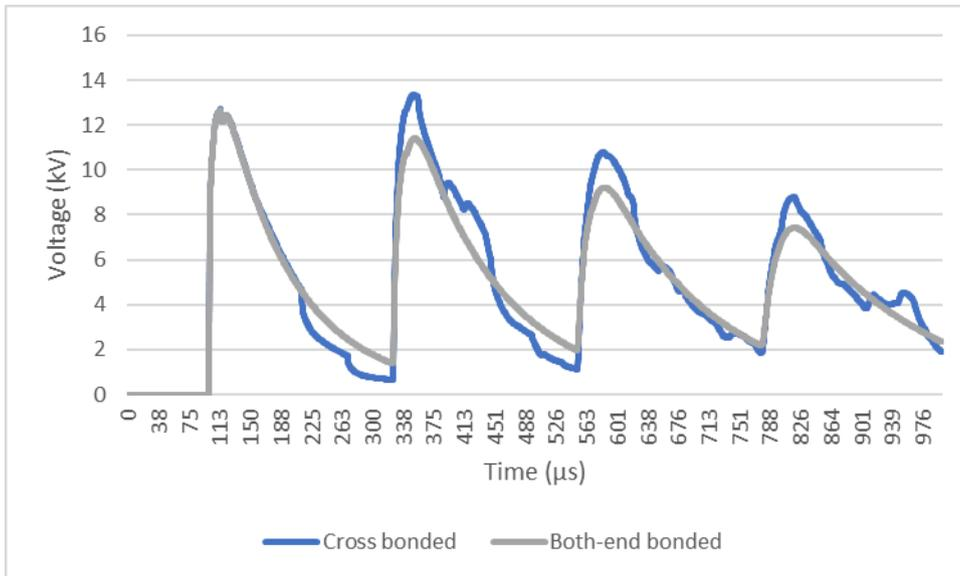
Figure 6:23 Impact of cross-bonding on cable voltages: Grounding method | Short circuit
