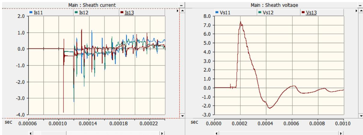
Figure 6:9 Sheath voltage and current in cable at the location of grounding in 'different location' grounding method
