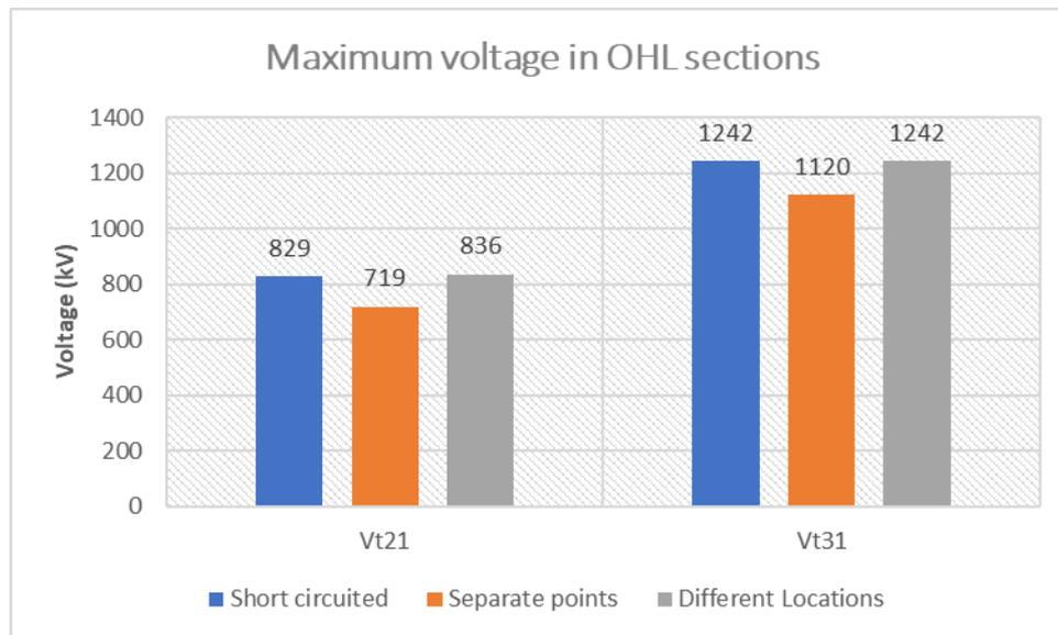
Figure 7:8 Comparison of maximum upper phase over voltage in OHL at tower 2 and 3: Lightning | Phase conductor
