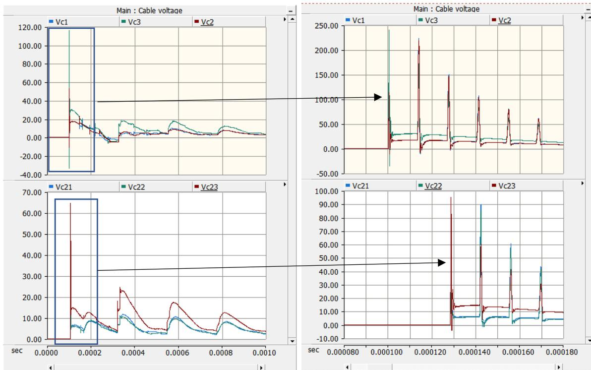
Figure 6:7 Overvoltage and current in cable: Lightning | Shield wire; Grounding Configuration | 'different location' ; Sheath | Both end bonded
