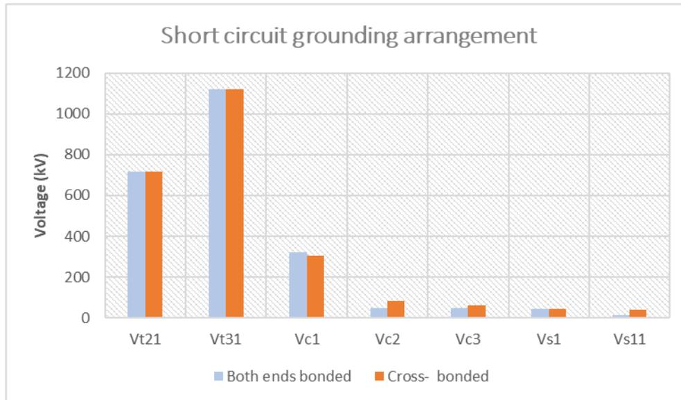
Figure 7:12 Impact of cross-bonding: Grounding method| Short circuit, Lightning| Phase conductor
