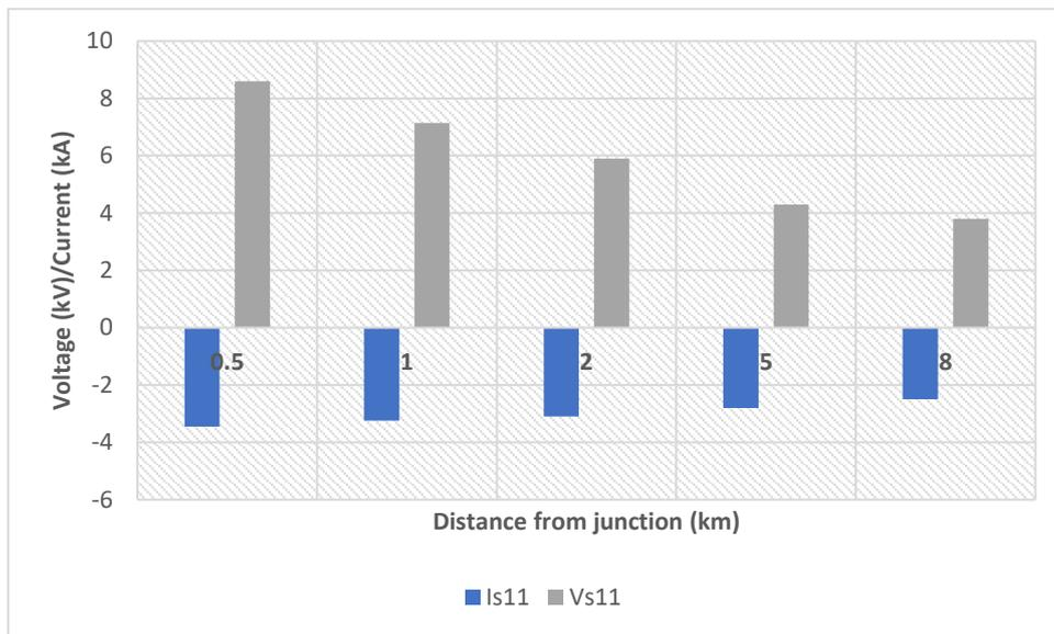
Figure 6:19 Sheath current and voltage change with distance
