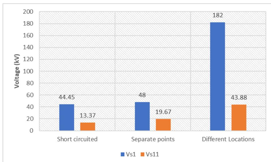
Figure 7:7 Variation of sheath voltage in different grounding schemes: Lightning| Phase conductor
