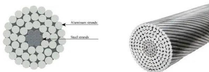
Figure 1:2 : ACSR conductor cross section on the left and ACSR strands on the right [8]
