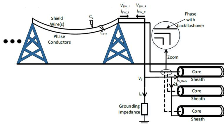
Figure 2:1 Lightning in Cable - OHL configurations [6]
