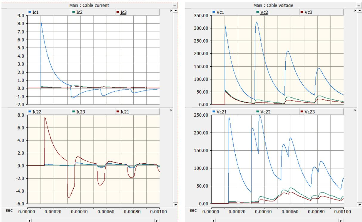
Figure 7:3 Overvoltage and current in cable: Lightning| Phase conductor; Grounding Configuration | 'separate points'
