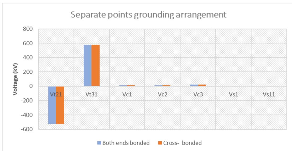
Figure 6:21 Impact of cross-bonding: Grounding method | 'separate points'
