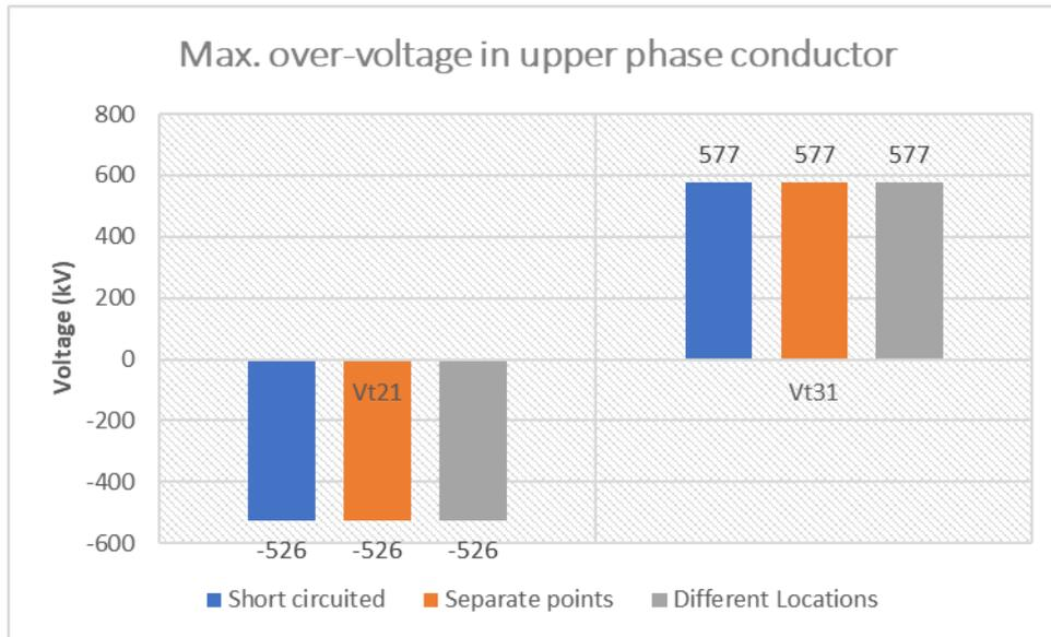
Figure 6:14 Comparison of maximum upper phase over voltage in OHL at tower 2 and 3: Lightning|Shield wire
