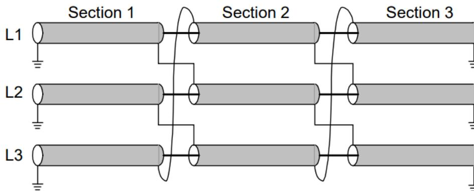
Figure 1:5 : Cross bonding in UGC [14]
