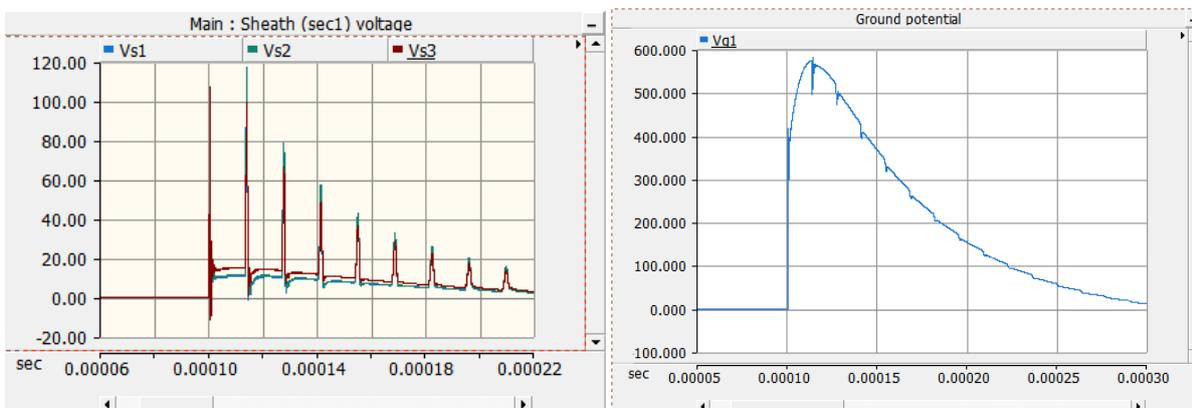
Figure 6:8 Ground potential and voltage induced in sheath at junction
