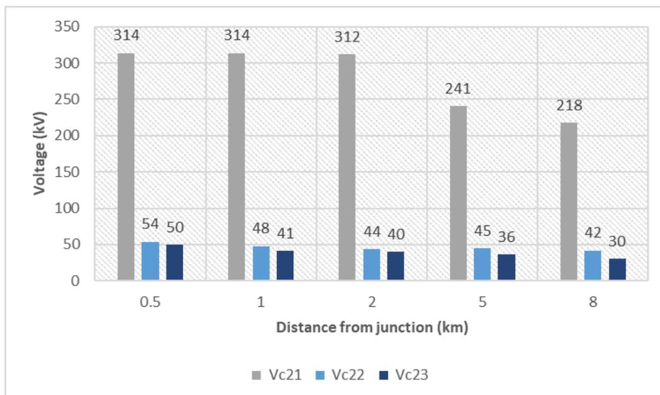
Figure 7:11 Impact of grounding location distance on cable: Lightning | Phase conductor
