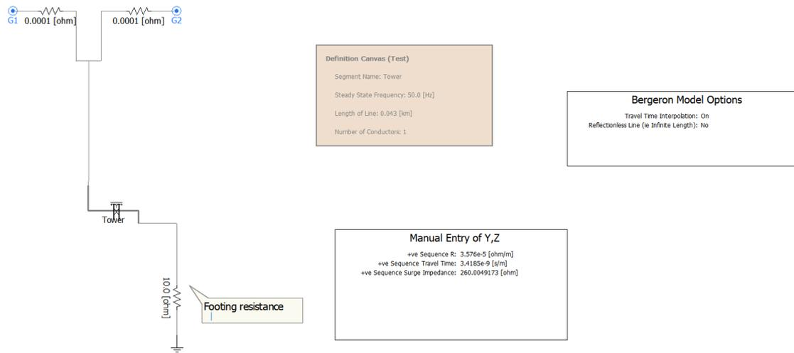
Figure 5:3 PSCAD Tower Model
