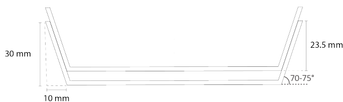
III. 79. Initial testing of the stackable principle (bottom)
