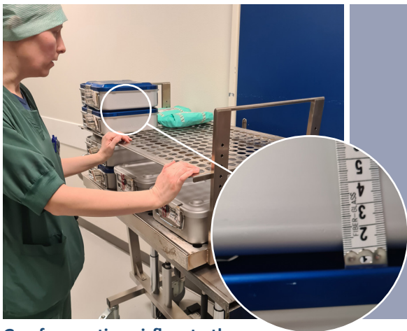
Gap for creating airflow to the filter was measured to 1 cm.
