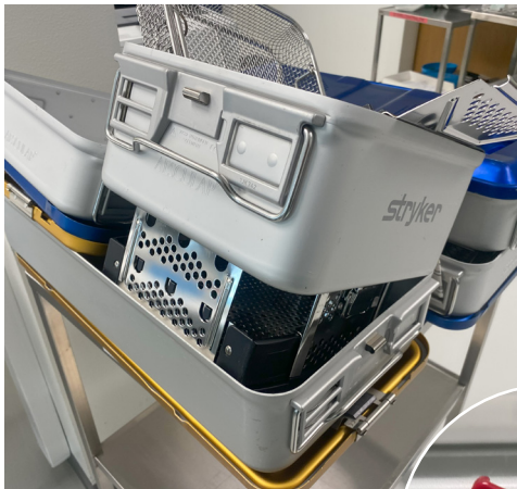
Visible indicators on the seal and filter show whether the container has been autoclaved.
