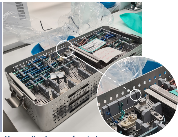
Air gap allowing a surface to be sterilised was measured to 2 mm
