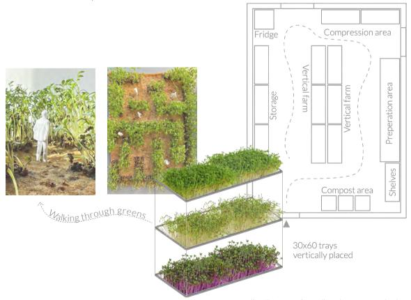
Illu. 47: Layout of a smaller microgreen production
