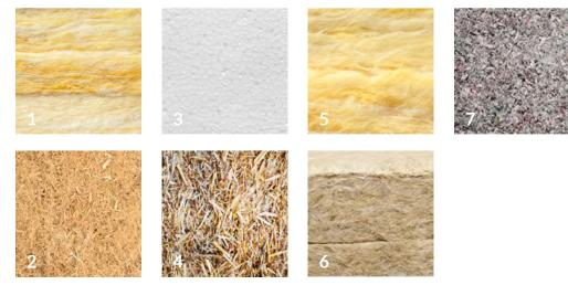
1: Mineral wool, 2: Wood fiber, 3: EPS insulation, 4: Straw, 5: Mineral wool, 6: Rock mineral wool, 7: Cellulose
