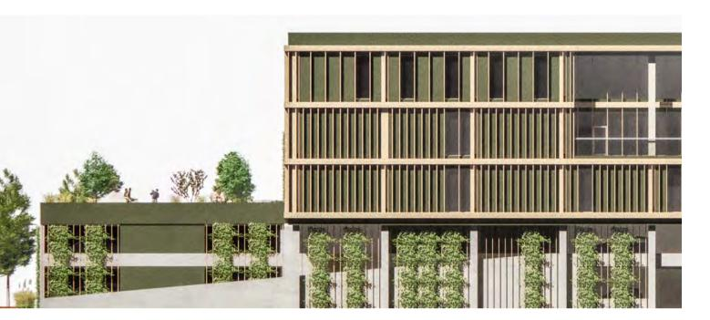
The eastern elevation has fenestration over the parking ramps which contributes to a visual connection from visitors arriving by car to see into the green production. The northern façade creates a tucked-in covered roof terrace, which lightens the otherwise closed façade. The fenestrations in the building adjust to the slats which emphasize a clean and symmetric rhythm in the lines of the frames of the façade.
