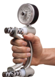
Figure 7 shows a Jamar Plus+ hydraulic hand dynamometer.
