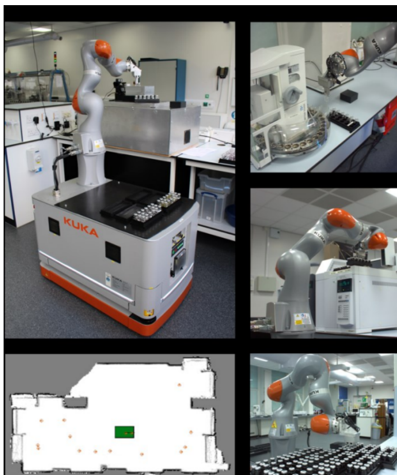
Figure 2.5: The KMR iiwa platform is used to automate chemical experimentation by going to different pre-defined locations, shown in orange on the map. The locations correspond to different stations used for dispensing, loading, storing, etc.[14]
