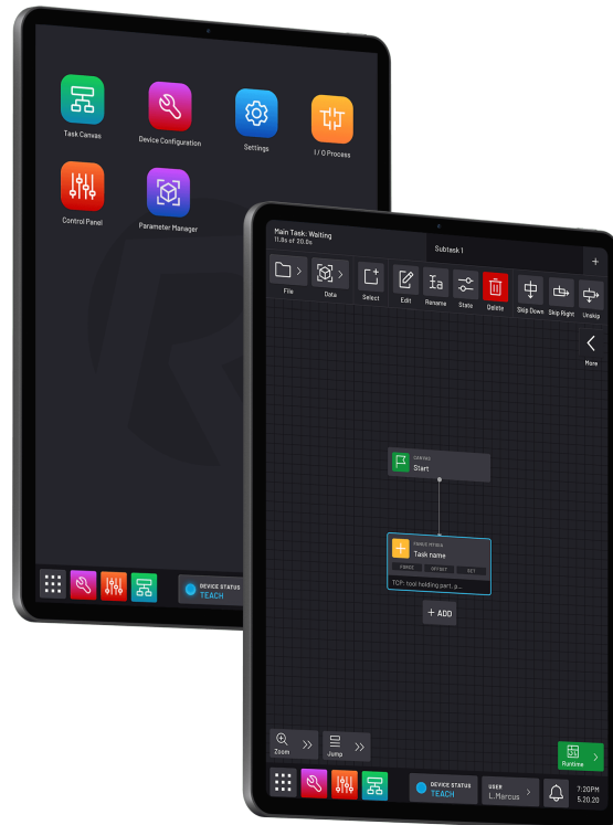
Figure 2.11: Image showing the user interface of ForgeOS developed by Ready Robotics, which uses finite-state-machines for programming of robots and supports a large variety of robot manufacturers [20]
