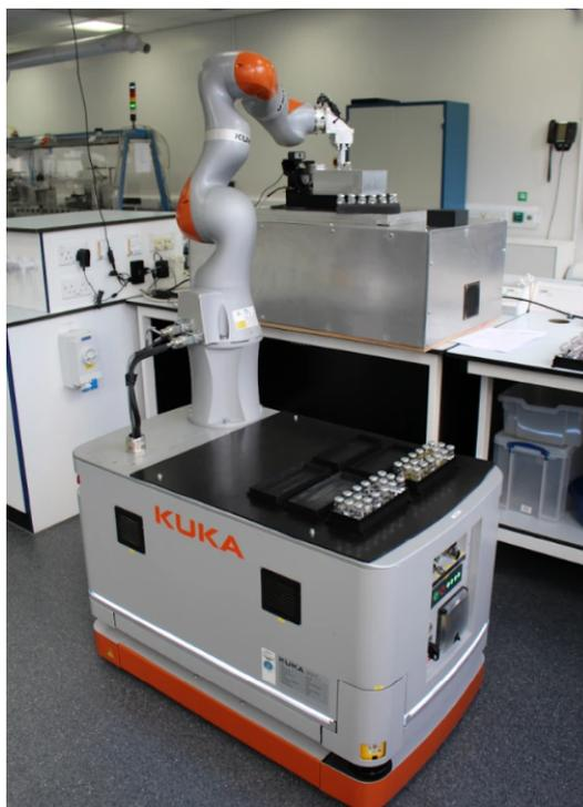
**Figure 2.10:** The Kuka mobile chemist platform. Reproduced from Burger et al [16], with permission from Springer Nature.
