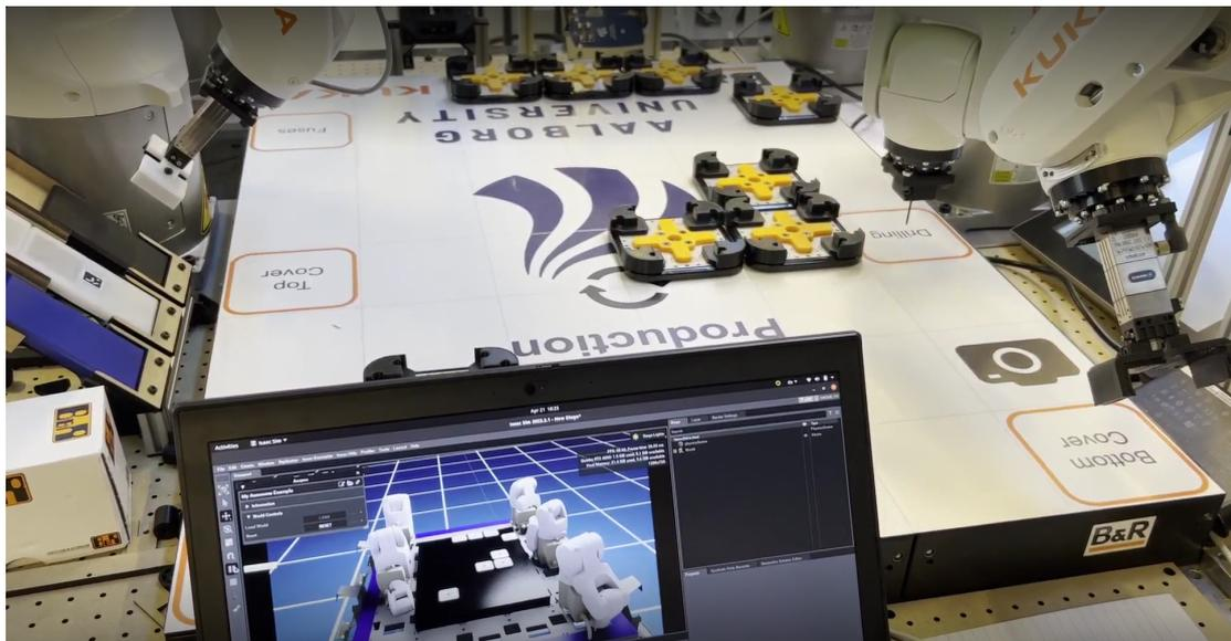
Figure 5.5: Testing the control of the Acopos 6D platform from the simulation environment in Isaac Sim.
