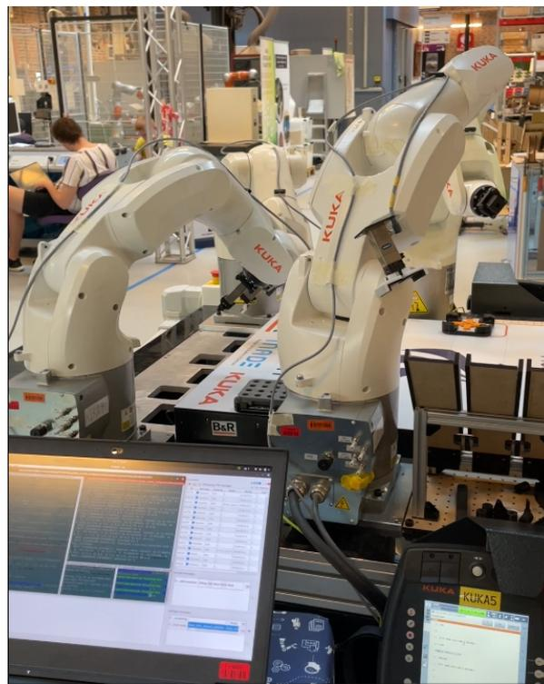
**Figure 5.6:** Picture taken during the communication test between ROS and Kuka Kr3r540 robot.
