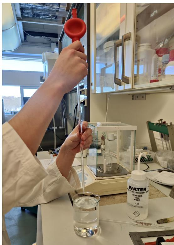
**Figure 2.19:** Extraction of exactly 5 ml of water with a precision pipette. It was observed that the collection process took on average more than 30 seconds.
