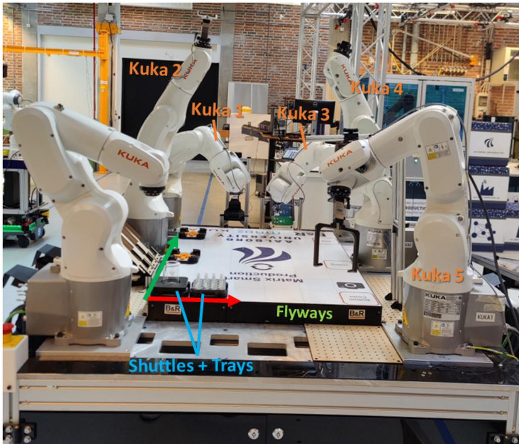
**Figure 4.22:** AAU Matrix Production Setup. The kuka manipulator arms used can be observed. Kuka 5 is the only Kuka KR4 R600, the others are Kuka KR3 R540. The red and green arrows show the x and y axes of the Acopos 6D platform respectively, which is composed of 12 flyways.
