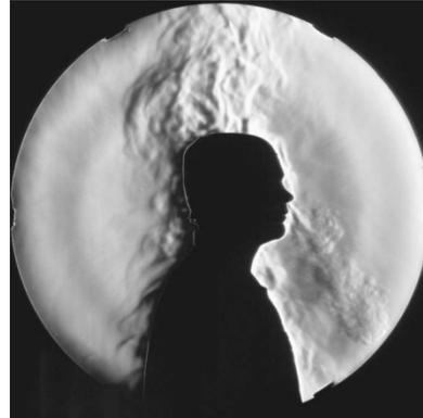
**Figure 1** Convective boundary layer of a human. The thermal plume can be seen above the head.[Craven and Settles, 2006]
