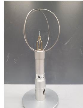
**Figure 1.21** Danvak 54R102 thermal comfort probe
