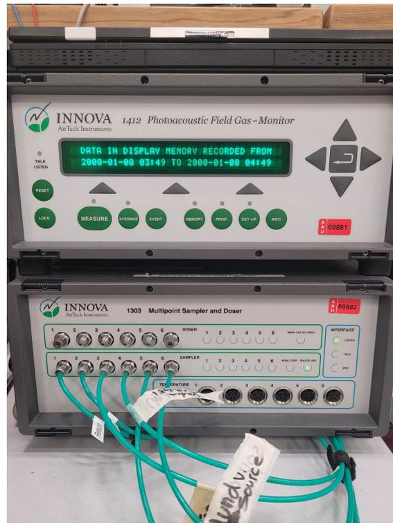
**Figure 1.24** Photoacoustic field gas monitor and multipoint sampler and doser.
