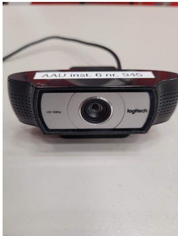
**Figure 1.25** Video camera used for smoke measurements.
