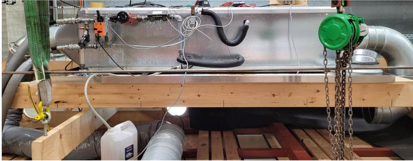
**Figure 1.6** AHU used for ventilation of the room. The intake is under the AHU on the right side.
