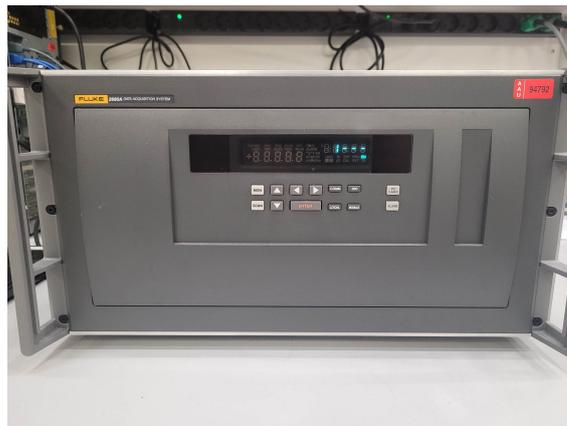
**Figure 1.19** Helios datalogger
