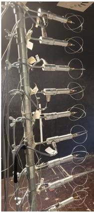
**Figure 1.22** Position of anemometers during measurements of the velocity profile.
