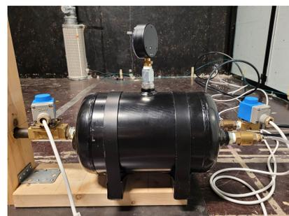
**Figure 1.14** Coughing machine seen from the side. The outlet is on the left and the inlet is on the right.
