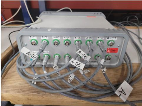
**Figure 1.20** Danvak datalogger for anemometers
