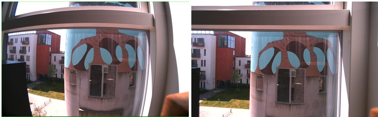
(a) Distorted image from the color imager. The wide lens increases the field of view but distorts the image. (b) Rectified image using the calibration supplied by Carnegie Robotics
