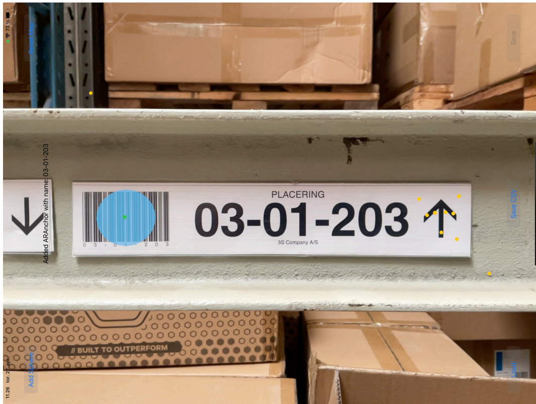
Figure 3.3: A screenshot of the test app showing blue spheres placed at the barcodes. Additionally, yellow dots can be seen, representing ARKit's features for tracking.
