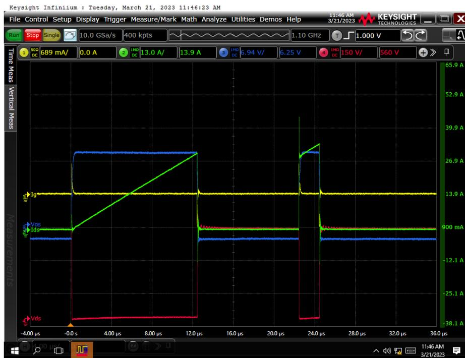
**Figure A.3:** Keysight PD1500A DPT waveforms for C3M0060065K measured at 30 A and 400 V.
