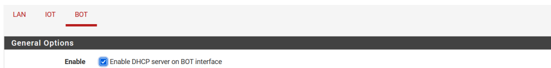
Figure 5.15: The DHCP configuration for the BOT interface.
