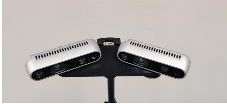
**Figure 4.5:** Mounting bracket for two *RealSense* cameras
