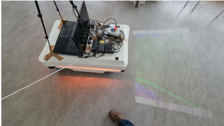
**Figure 1.1:** A projector used to show the planned path of the robot on the floor. This is used to highlight the intended action of the robot to the user.
