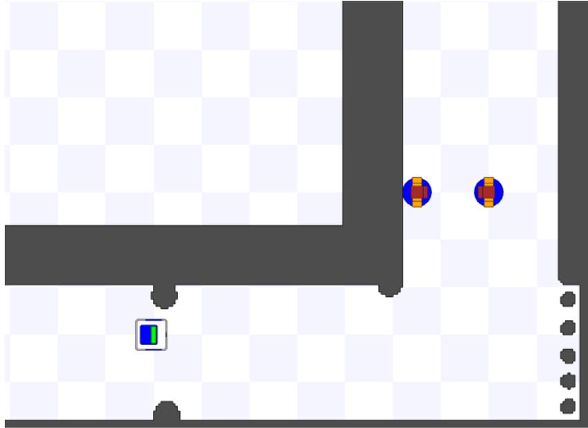
**Figure 5.1:** An example of the test environment. The environment contains walls (grey), a simulated robot (white, blue and green box) and two humans (blue circles). The location of people are published on the ROS network to be detected by the robot when planning movement.
