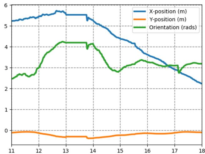
**Figure 5.10:** The performance of the People Detection Module when a person is further than 5m away and moving towards the robot. Here the blue graph is the X-position in meters, orange is Y position in meters and green is the orientation in radians. The x-axis represents time in seconds.
