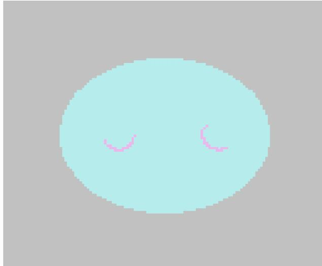
**Figure 4.13:** An example of the costmap of an interaction zone of two people, visualised in RViz. The location of the two people from the laser scan is shown with the two half circles in purple while the elliptical interaction zone is shown in turquoise. The constant colour represents the constant cost of the interaction zones.
