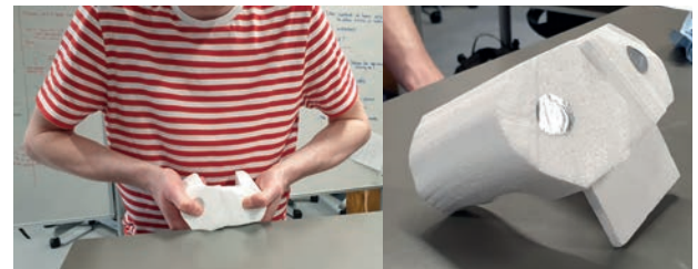
III. 130. "Model 1": A controller-like form with a dent that can be pressed against the table.
