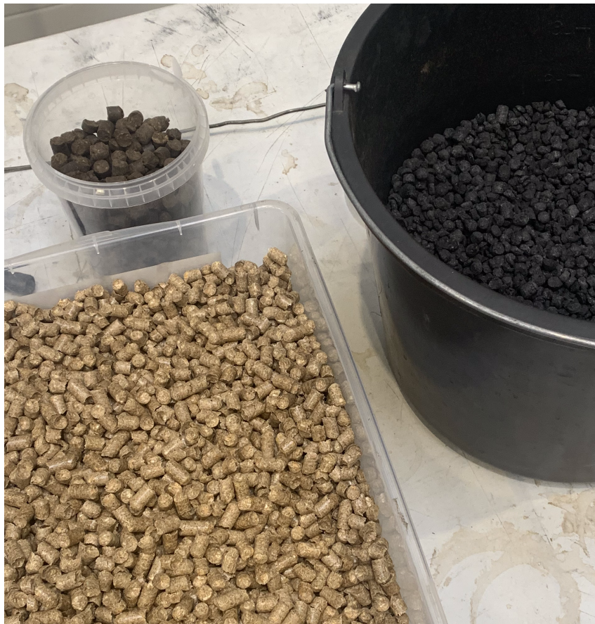
Figure 1.1. Pellets of straw (bottom left), biogas digestate (upper left) and biochar (right). Picture from Stiesdal SkyClean facility in GreenLab, Skive.
