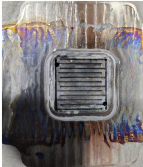
**Figure 4.23:** Bipolar plate from the anode side
