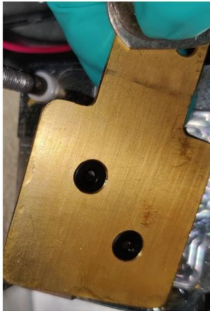
Figure 1.7: Current collector used in the laboratory
