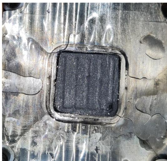
Figure 1.5: Membrane electrode assembly used in the laboratory
